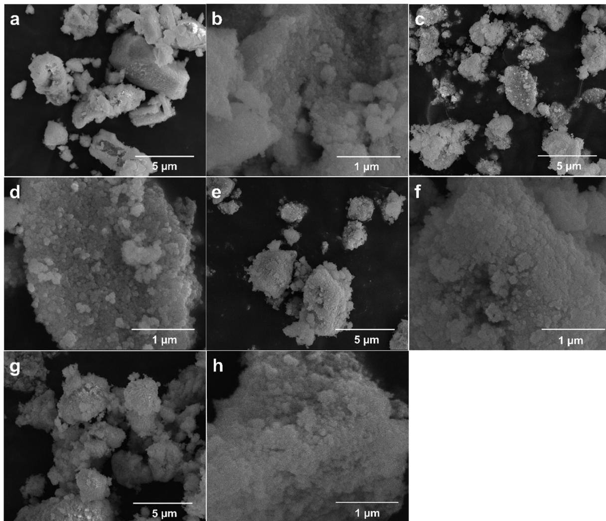
Fig. 2 SEM images of CeO<sub>2</sub> samples calcined under various conditions: Air450-1.4 (a) and (b), Air400-1.4 (c) and (d), Air450-5.0 (e) and (f), and Ar800-5.0\_Air450-1.4 (g) and (h).
