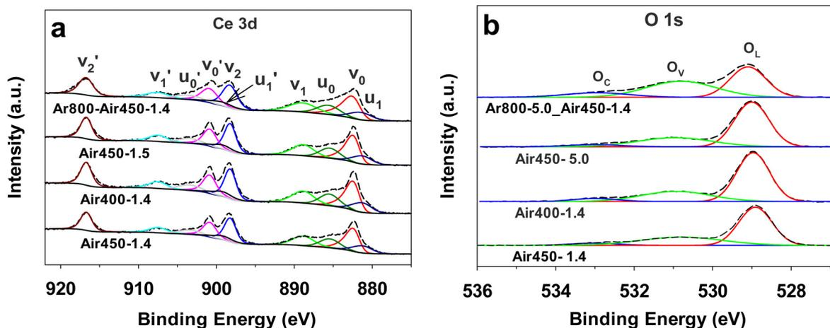
Fig. 6 Ce 3d XPS spectra (a) and O 1s XPS spectra (b) of CeO<sub>2</sub> samples calcined under various conditions.
