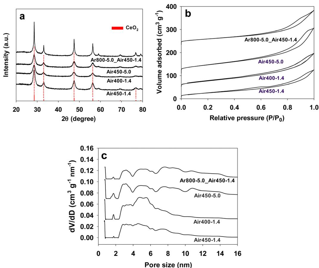
Fig. 1 XRD patterns (a), nitrogen adsorption isotherms (b), and pore size distributions (c) of CeO<sub>2</sub> samples prepared under various calcination conditions which are indicated in their names.
