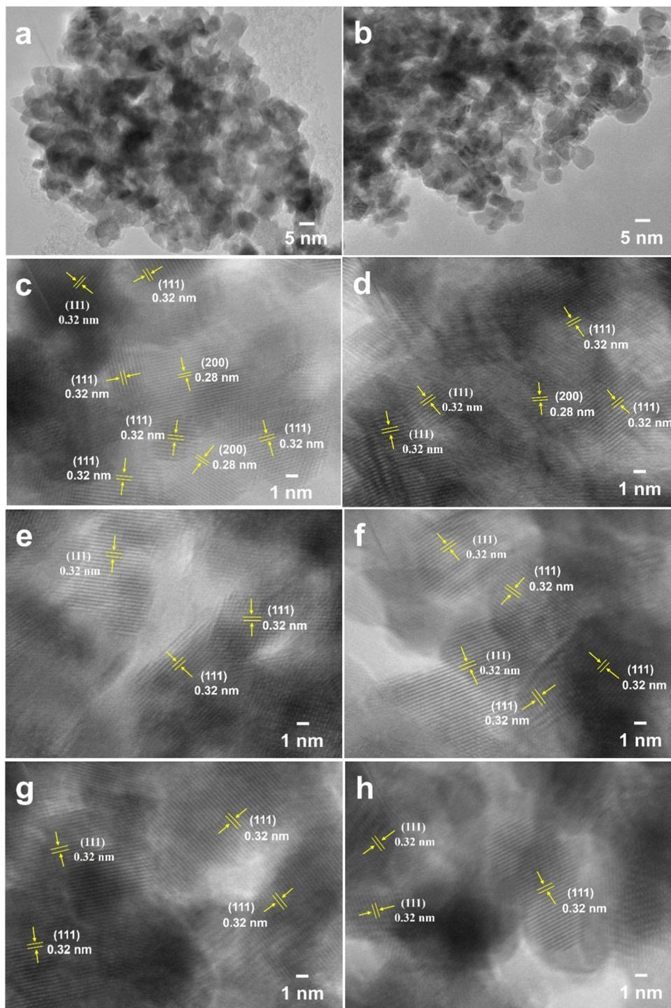
Fig. 3 TEM images of CeO<sub>2</sub> samples Air450-1.4 obtained *via* one-step calcination (a), (c), (e) and (g) and Ar800-5.0\_Air450-1.4 obtained *via* two-step calcination (b), (d), (f) and (h).
