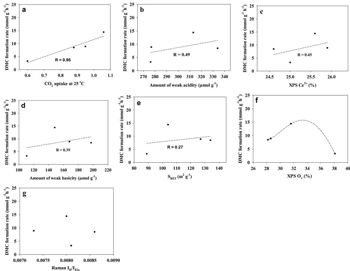
Fig. 7 Effect of various parameters of CeO<sub>2</sub> samples on the DMC formation rate: (a) CO<sub>2</sub> uptake at 25 °C, (b) amount of weak acidity (NH<sub>3</sub> uptake at 100–300 °C), (c) XPS Ce<sup>3+</sup>%, (d) amount of weak basicity (CO<sub>2</sub> uptake at 100–300 °C), (e) BET surface area (S<sub>BET</sub>), and (f) XPS O<sub>1s</sub>%, and (g) Raman peak intensity ratio I<sub>D</sub>/I<sub>F<sub>2g</sub></sub>.
