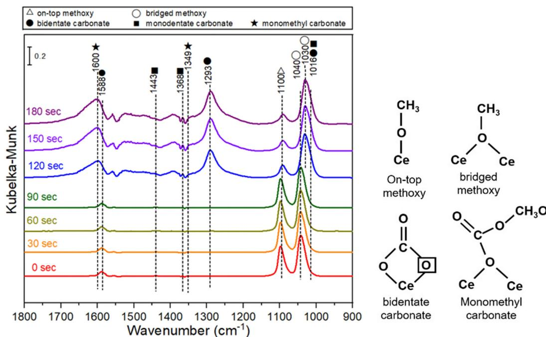
Fig. 8 *In situ* DRIFTS spectra of CeO<sub>2</sub> (Air450-1.4) with pre-adsorbed methanol followed by purging CO<sub>2</sub> at 140 °C.
