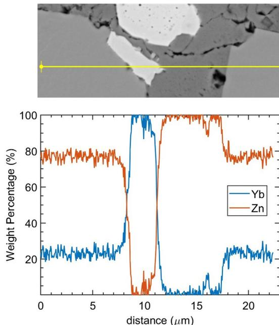
Fig. 4 EDS line scan on the defect site. The scanning line goes through the YbZn<sub>11</sub> matrix, Yb oxides (white), Zn-rich phase (dark grey), and YbZn<sub>11</sub>.
