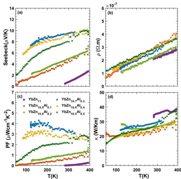
Fig. 8 (a) Seebeck coefficient, (b) resistivity, (c) power factor, and (d) thermal conductivity of  $\text{YbZn}_{11-x}\text{Al}_x$  samples ( $x = 0, 0.1, 0.2, 0.3, 0.4, 0.5$ ) *versus* temperature from 70–400 K.
