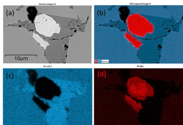
**Fig. 3** EDS mapping. (a) BSE image of a typical defect site with cavities (black), Yb oxides (white), Zn (dark grey), and compared to YbZn<sub>11</sub> (light grey). (b) layered EDS map, (c) Zn distribution EDS map, and (d) Yb distribution map. The blue and red dots in (c) and (d) represent the relative Zn and Yb concentration.
