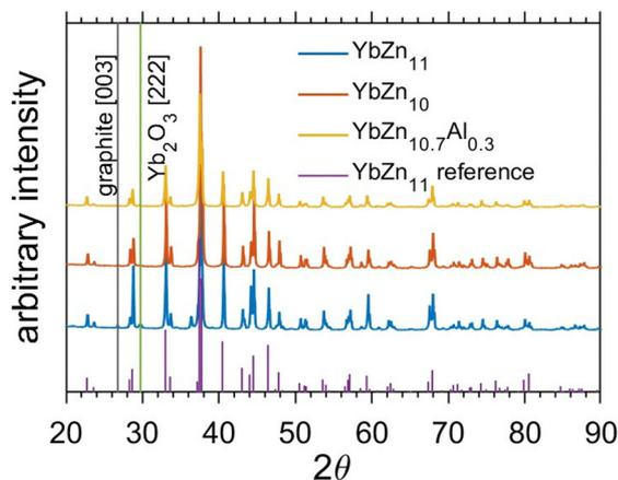
**Fig. 1** XRD results of Yb–Zn samples, the annealed intrinsic YbZn<sub>11</sub> sample in blue, the Zn-deficient sample YbZn<sub>10</sub> sample in orange, and the Al-substitution sample YbZn<sub>10.7</sub>Al<sub>0.3</sub> in yellow, and the reference peaks in purple.<sup>28</sup> Minor impurity peaks from graphite and ytterbium oxide are marked by black and green lines.
