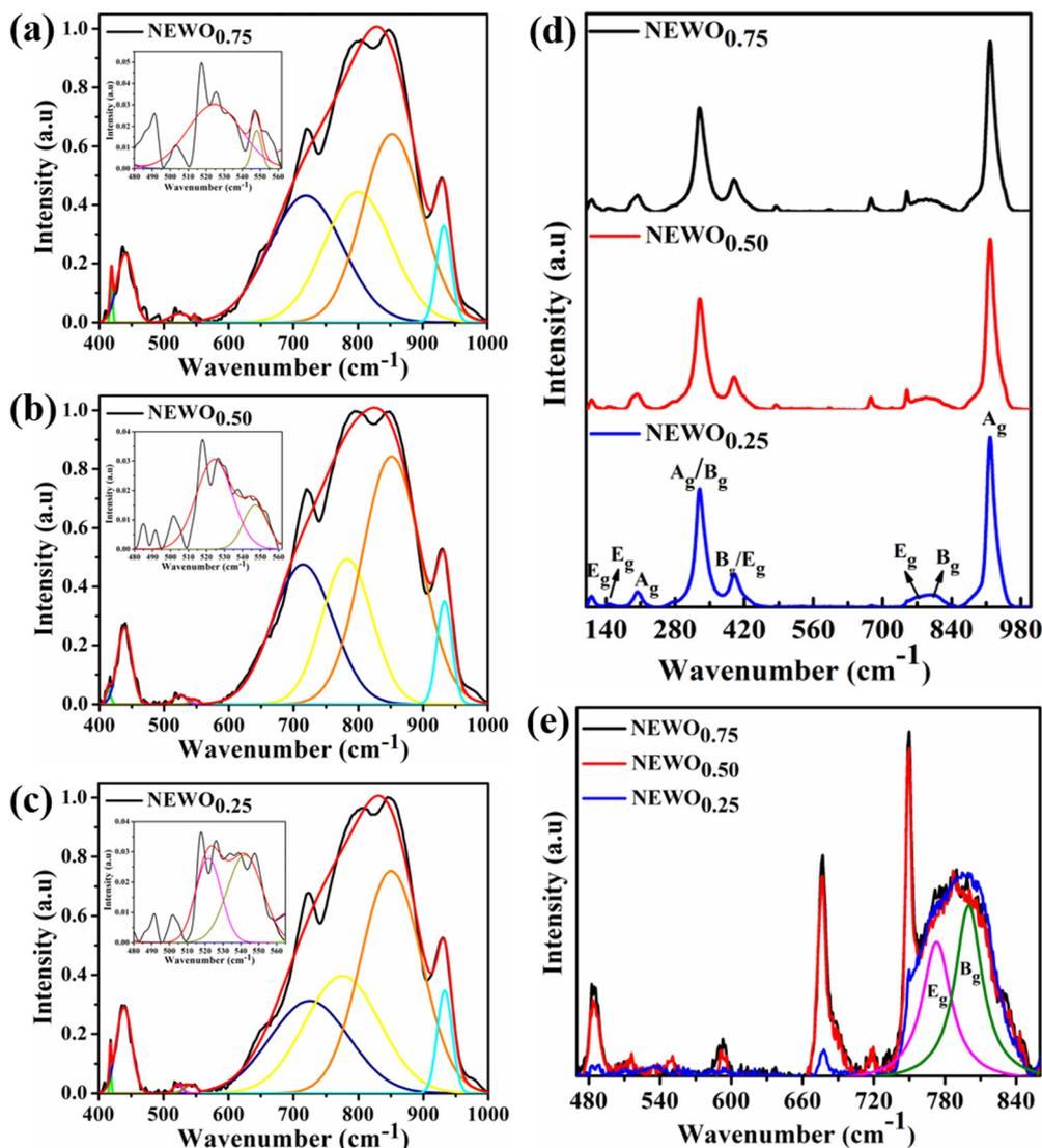
Fig. 3 Deconvoluted peaks of the FTIR spectrum: (a)  $\text{NEWO}_{0.75}$ , (b)  $\text{NEWO}_{0.50}$ , and (c)  $\text{NEWO}_{0.25}$ . (d) Raman spectra of  $\text{NEWO}_{0.75}$ , and  $\text{NEWO}_{0.50}$ ,  $\text{NEWO}_{0.25}$ . (e) Magnified Raman spectra ( $480\text{--}840\text{ cm}^{-1}$ ).
