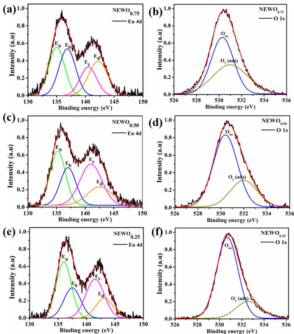
Fig. 4 High-resolution XPS spectra of the Eu 4d state and O 1s state of (a) and (b) NEWO<sub>0.75</sub>. (c) and (d) NEWO<sub>0.50</sub> and (e) and (f) NEWO<sub>0.25</sub>.
