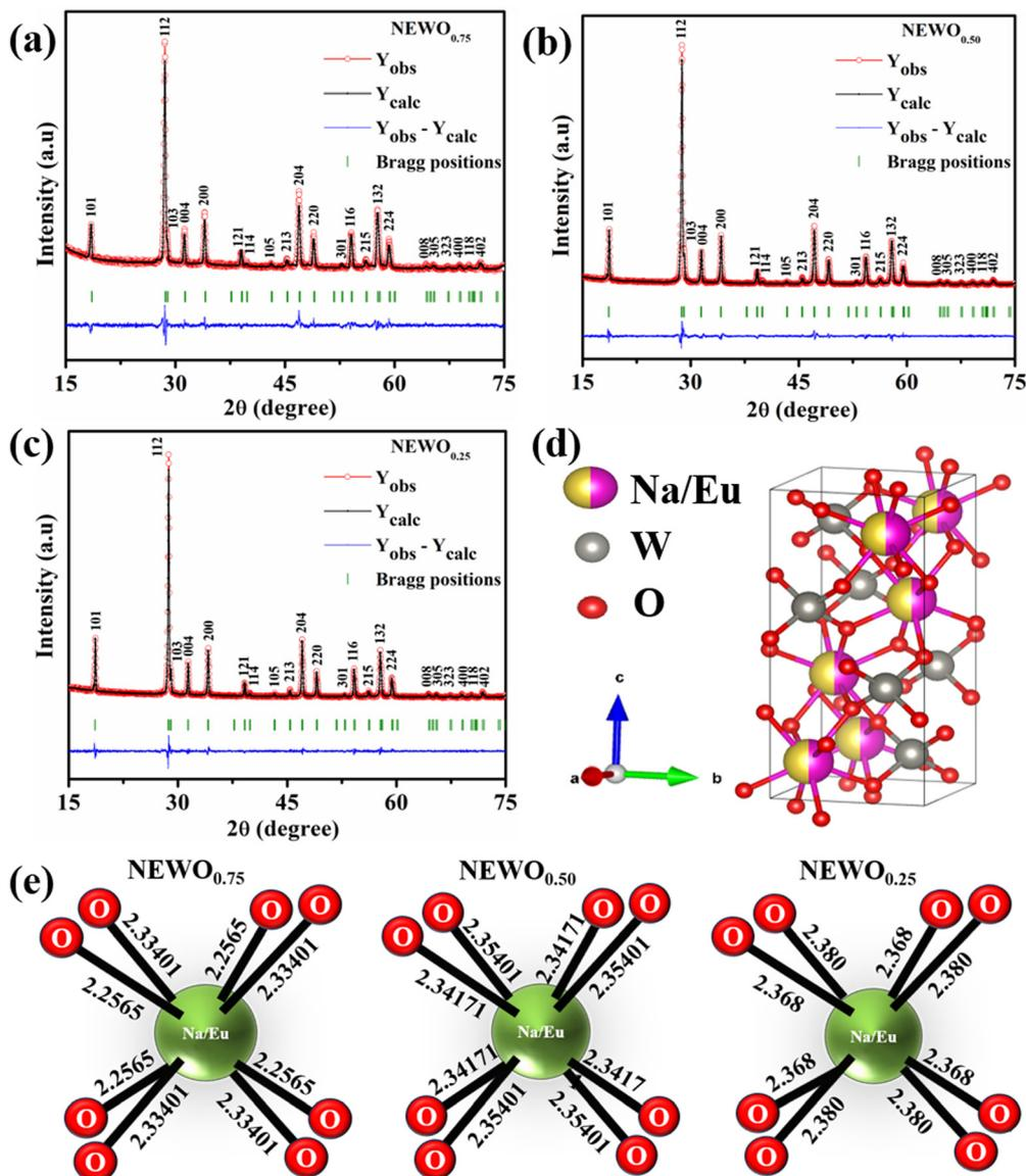
Fig. 1 The observed and refined XRD pattern of  $\text{NaEu}(\text{WO}_4)_2$  samples: (a)  $\text{NEWO}_{0.75}$ , (b)  $\text{NEWO}_{0.50}$ , (c)  $\text{NEWO}_{0.25}$ , (d) unit cell of the  $\text{NaEu}(\text{WO}_4)_2$  tetragonal structure and (e) the schematic representation of the variation in the bond lengths of the  $\text{Na/Eu-O}$  dodecahedron in  $\text{NaEu}(\text{WO}_4)_2$ .
