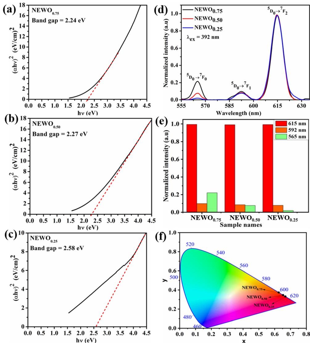
Fig. 5 Tauc plot: (a) NEWO<sub>0.75</sub>, (b) NEWO<sub>0.50</sub>, and (c) NEWO<sub>0.25</sub>. (d) PL spectra of NEWO<sub>0.75</sub>, NEWO<sub>0.50</sub>, and NEWO<sub>0.25</sub>. (e) Bar diagram of the normalized PL intensity of samples and (f) CIE diagram of NEWO<sub>0.75</sub>, NEWO<sub>0.50</sub>, and NEWO<sub>0.25</sub> samples.
