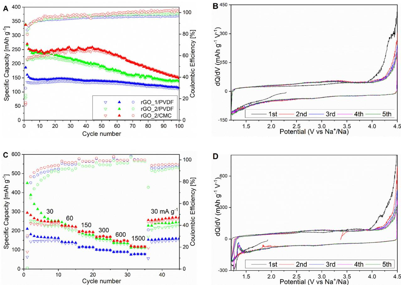
**Fig. 3** Electrochemical performance of two rGO cathodes. (A) Galvanostatic cycling of rGO\_1 and rGO\_2 cathodes with PVDF binder and rGO\_2 with CMC binder. The electrodes were cycled at 30 mA g<sup>-1</sup> in 1.2–4.5 V voltage window. (B) and (D) The extracted dQ/dV vs. V curves of first 5 cycles of cathodes rGO\_1/PVDF (B) and rGO\_2/PVDF (D). (C) Rate capability of rGO\_1 and rGO\_2 cathodes with PVDF binder and rGO\_2 with CMC binder. Legend as in (A).
