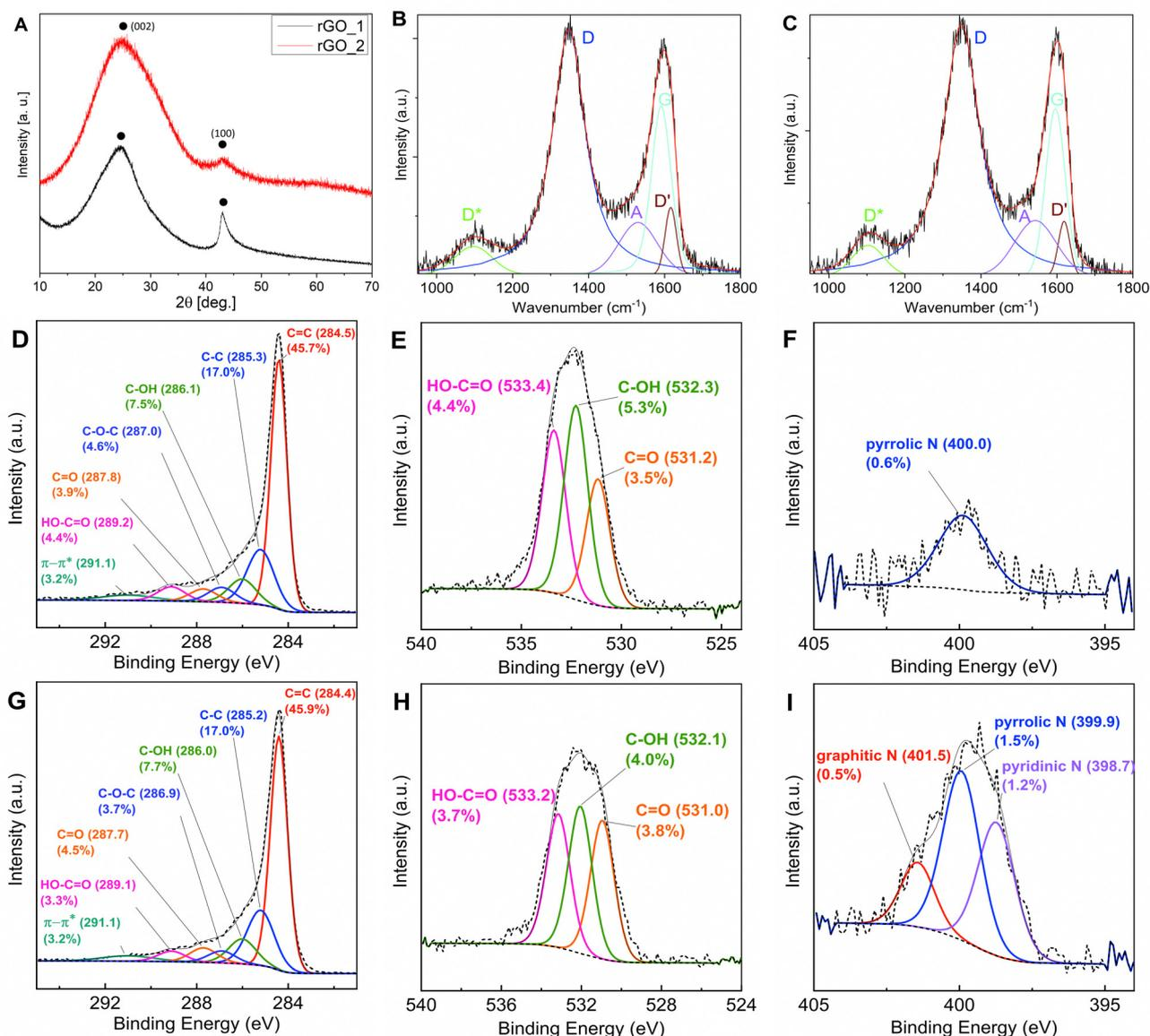
**Fig. 1** Characterization of two different rGO materials, (A) X-ray diffraction pattern of rGO\_1 and rGO\_2 (black dots indicate peaks of rGO). (B) and (C) Raman spectrum of rGO\_1 (B) and rGO\_2 (C) in G and D bands region with 5 fitted peaks. (D)–(F) XPS spectra of rGO\_1 in the C 1s region (D), O 1s region (E) and N 1s region (F). (G)–(I) XPS spectra of rGO\_2 in the C 1s region (G), O 1s region (H) and N 1s region (I).
