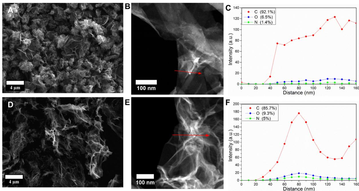
Fig. 2 Electron microscopy characterization of two different rGO materials. (A), (B), (D), (E) SEM and high-angle annular dark-field STEM images of rGO<sub>1</sub> (A), (B) and rGO<sub>2</sub> (D), (E) samples. (C), (F) The corresponding TEM EDX line scans of rGO<sub>1</sub> (C) and rGO<sub>2</sub> (F). Red arrow indicates the path of line scan.
