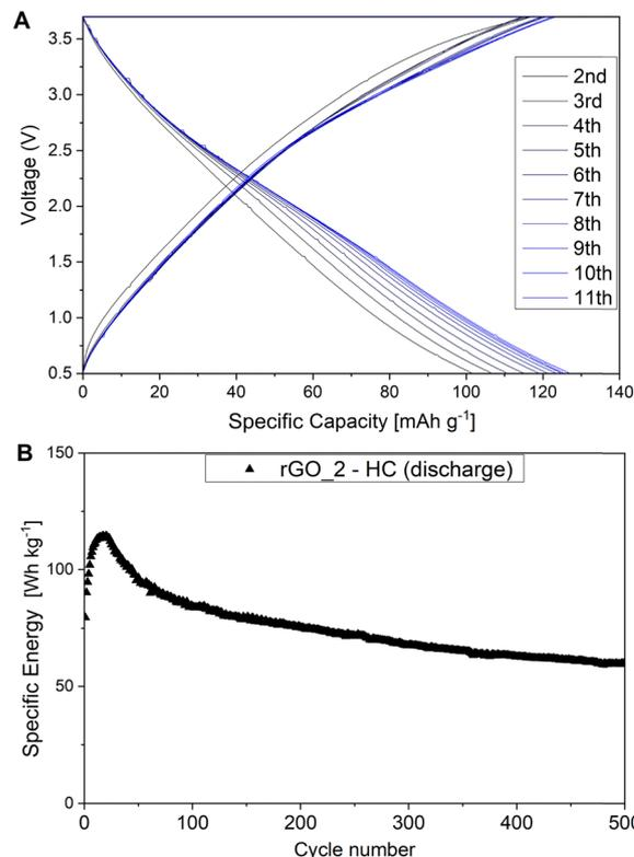
**Fig. 7** Electrochemical performance of all carbon full cell. (A) Voltage profiles of first of rGO\_2/CMC – HC full cell cycled in 0.5–3.7 V voltage window. (B) Energy density performance of full cell during long galvanostatic cycling.
