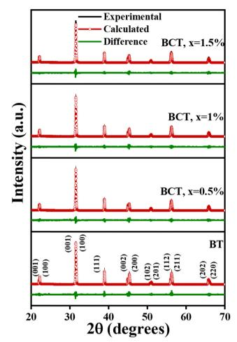
Fig. 2 Rietveld refined XRD patterns of BT and BCT ceramics.
