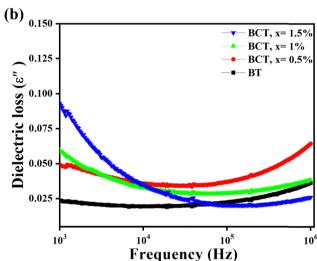
Fig. 7 Variation of the (a) dielectric constant and (b) dielectric loss of BT and BCT ceramics with varying frequencies.
