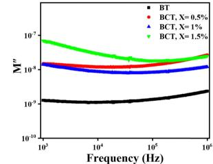
Fig. 9 Variation of the (a) real component of the dielectric modulus (M')and (b) imaginary component of the dielectric modulus (M") with frequency.
