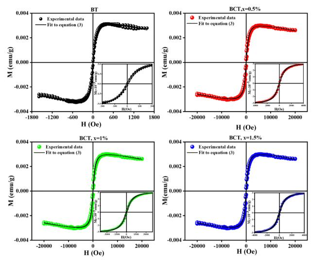
Fig. 6 M-H curves of (a) BT and (b)-(d) BCT ceramics (0.5, 1, and 1.5 mol%) at room temperature. The insets at the right bottom corner show the magnified snapshots near the origin. The black solid line overlapping the data points represents the fitting of the M-H loop by using eqn (3).
