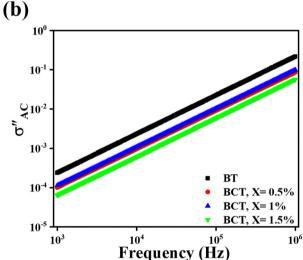
Fig. 8 Variation of (a) the real part of AC conductivity (the inset image shows the variation of the frequency exponent s with Ce concentration) and (b) the imaginary part of AC conductivity of BCT ceramics against frequency.
