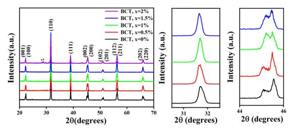
Fig. 1 XRD patterns of BT and BCT ceramics with x = 0.5%, 1%, 1.5% and 2% (left); shift of the peaks at 31° (center) and 45° (right) on cerium doping.
