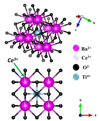
Fig. 3 Crystal structures of BT and BCT ceramics generated using Vesta software using Rietveld refined structural parameters
