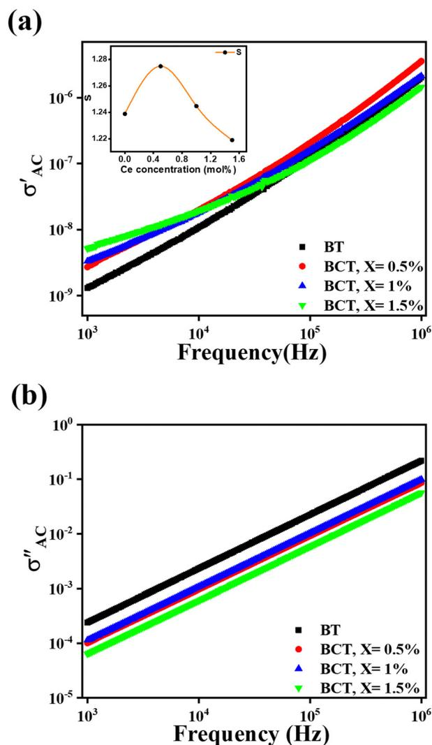
**Fig. 8** Variation of (a) the real part of AC conductivity (the inset image shows the variation of the frequency exponent  $s$  with Ce concentration) and (b) the imaginary part of AC conductivity of BCT ceramics against frequency.
