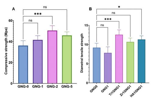
Fig. 7 (A) Compressive strength of ionogel modified glass ionomer cement (GNG) at different weight percentages of ionogel in the polyalkenoic acid formulation. (B) Diametrical tensile strength of the ionogel modified glass ionomer cement (GNG1) with 1 wt% TiOH (TiIGNG1), HA (HAIGNG1), and ZrOH (ZrIGNG1).
