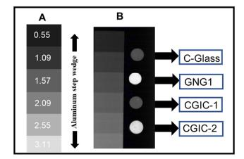
Fig. 9 (A) Different thickness (mm) of aluminum step wedge. (B) Radio-opacity of the aluminum step wedge, C-glass (GIC prepared using commercial glass and in-house polymer), GNG1 (in-house GIC with 1% ionogel), and CGIC-1 and CGIC-2 as different commercial GIC samples as controls.
