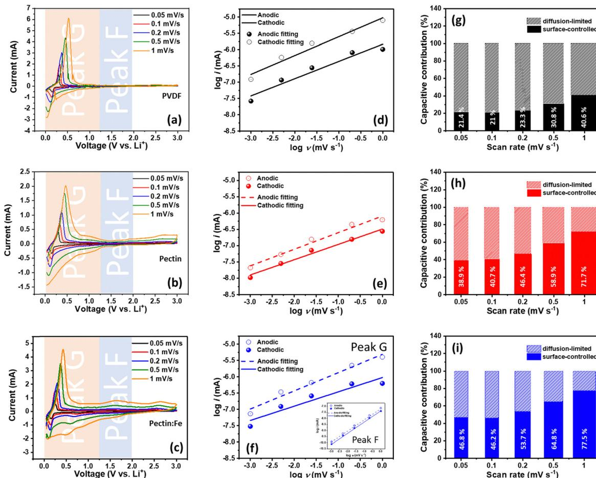
Fig. 1 CV curves for (a) graphite–PVDF, (b) graphite–pectin, and (c) graphite–pectin:Fe electrodes at different voltage scan rates, ranging from 0.05 to 1 mV s<sup>-1</sup>. Determination of the *b* value for (d) graphite–PVDF, (e) graphite–pectin, and (f) graphite–pectin:Fe electrodes using the relationship between the peak current and sweep rate. (g)–(i) show the percentage of capacitive contribution at different voltage scan rates for all the samples.
