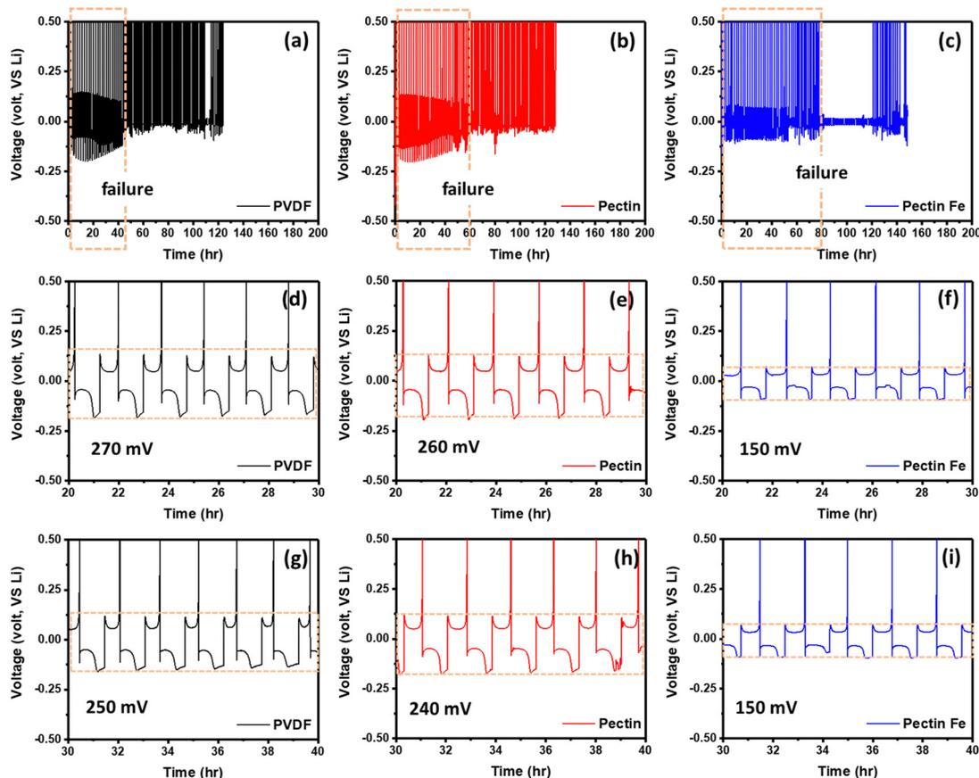
Fig. 4 Voltage profiles of the Li plating/stripping process for (a) PVDF, (b) pectin, and (c) pectin:Fe electrodes. Selected magnified voltage–time profiles of PVDF, pectin, and pectin:Fe electrodes are shown in (d)–(i).
