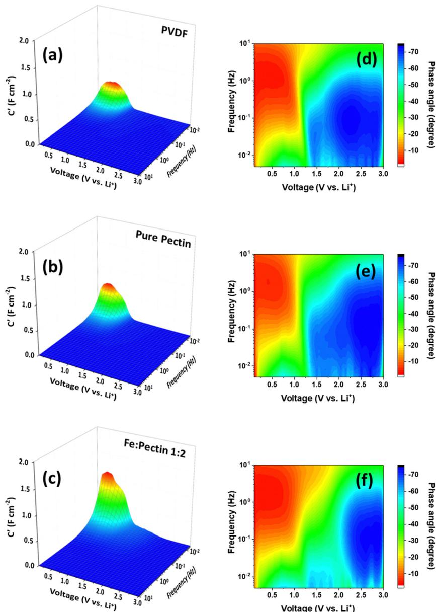
Fig. 2 3D Bode plots representing the real area-normalized capacitance ( $C'$ ) versus frequency versus voltage for (a) PVDF, (b) pectin, and (c) pectin:Fe. The corresponding representations of the phase angle ( $\phi$ ) versus frequency and voltage are shown for (d) PVDF, (e) pectin, and (f) pectin:Fe.
