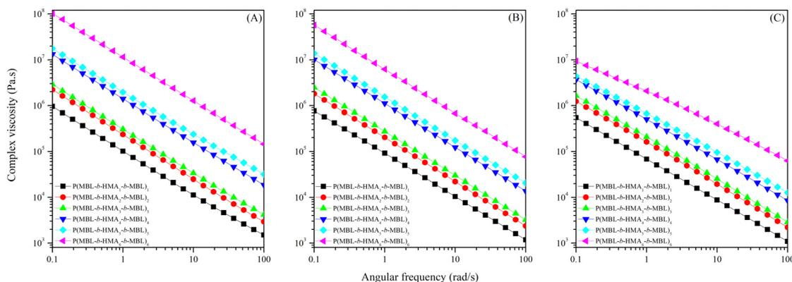
Fig. 3 Frequency sweep of the P(MBL-*b*-PHMA<sub>*x*</sub>-*b*-PMBL)<sub>*x*</sub> terblock copolymers at different temperatures (A) 110 °C, (B) 160 °C, (C) 200 °C.
