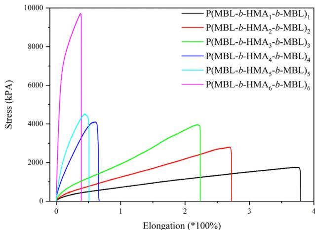
Fig. 4 Stress–strain curve of the  $P(\text{MBL-}b\text{-HMA}_x\text{-}b\text{-MBL})_x$  terblock copolymers.
