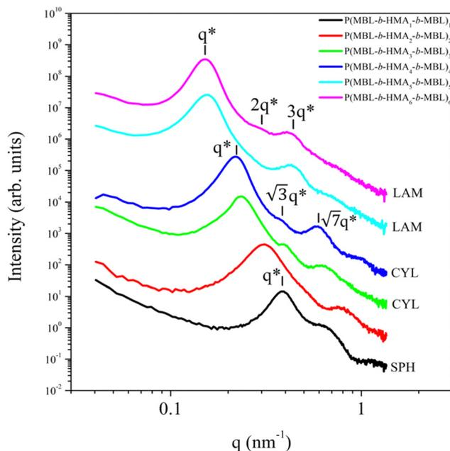
**Fig. 2** SAXS curves for the P(MBL-*b*-PHMA<sub>*x*</sub>-*b*-PMBL)<sub>*x*</sub> terblock copolymers.
