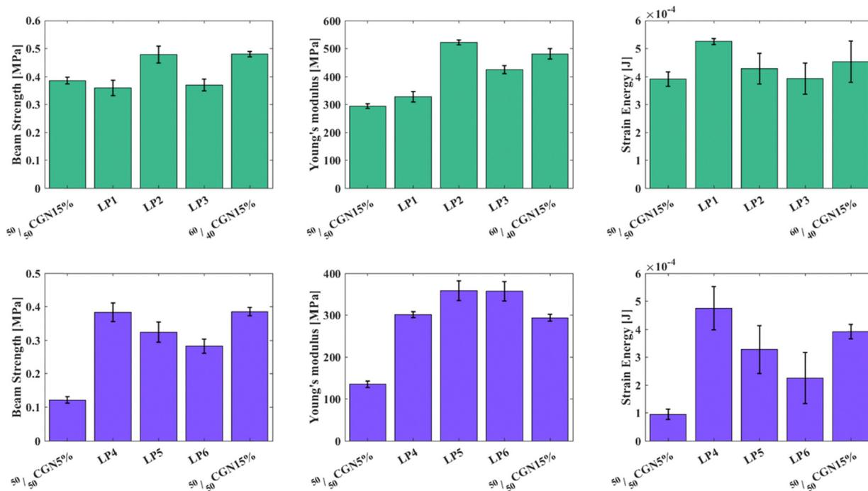
Fig. 4 Mechanical properties of *O. wendtii* (A)–(C) and *O. scyllarus* (D)–(F) inspired models. (A) BST measurements (B) Young modulus and (C) strain energy graphs of 50/50CGN15% and 60/40CGN15% models dispersed in various layered structures. (D) BST measurements (E) Young modulus and (F) strain energy graphs of 50/50CGN15% and 50/50CGN15% models dispersed in various layered structures.
