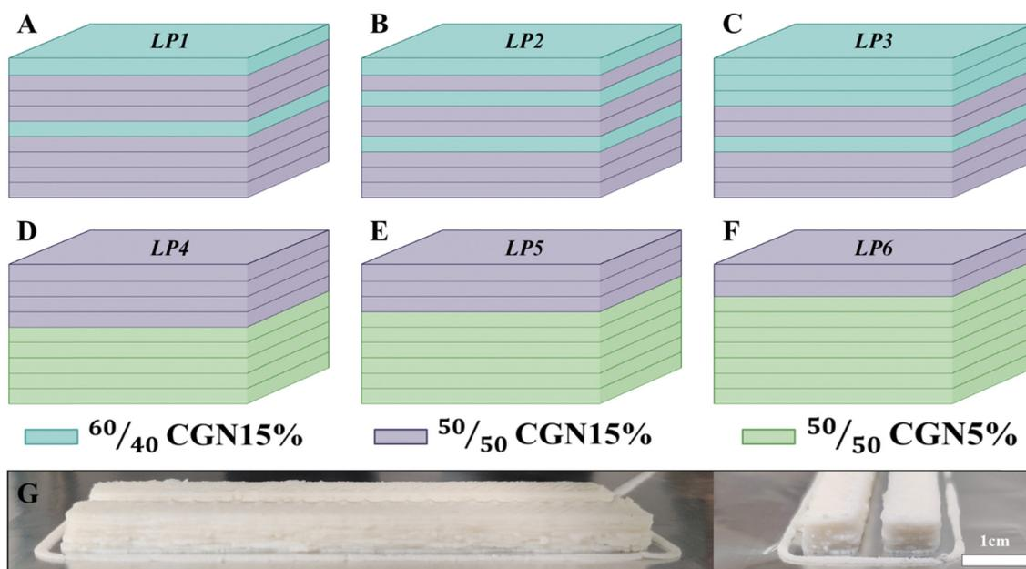
**Fig. 3** (A)–(C) 50/50CGN15% and 60/40CGN15% tested layered structures, inspired by the *O. wendtii* brittlestar. (D)–(F) 50/50CGN15% and 50/50CGN5% layered structure inspired by the *O. scyllarus* dactyl club (G) a printed sample.
