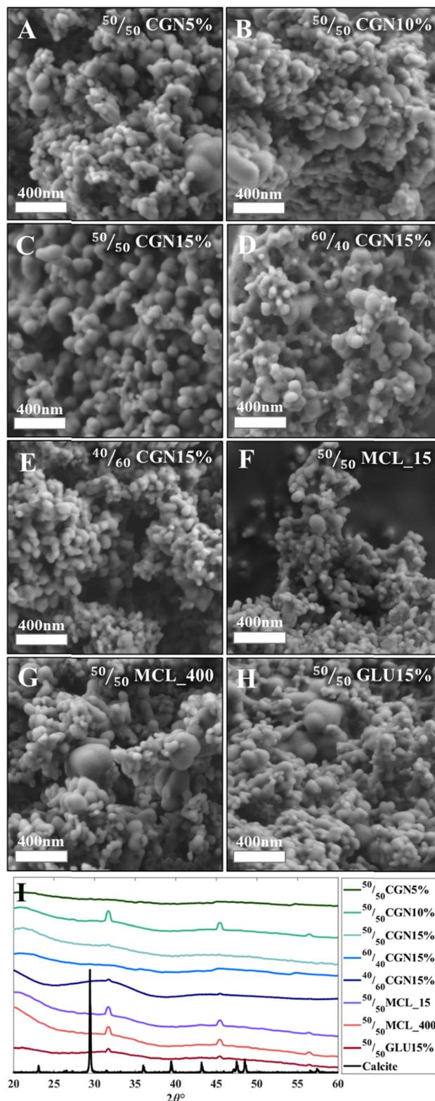
**Fig. 1** (A)–(H) HR-SEM images depict ACC 3D-printed models with various additives after sintering. ACC powders with additive-rich environments are shown as follows: (A) 50/50CGN5%; (B) 50/50CGN10%; (C) 50/50CGN15%; (D) 60/40CGN15%; (E) 40/60CGN15%; (F) 50/50MCL\_15; (G) 50/50MCL\_400 and (H) 50/50Glu15%. (I) HRPXRD patterns were collected at a wavelength of Cu K $\alpha$  1.546 Å and a wavelength of 0.3542 Å, normalized to Cu K $\alpha$ .
