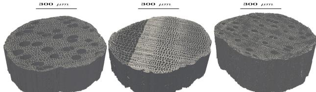
Fig. 1 The 3D scanned samples of poplar (left), spruce (middle), and maple (right)
