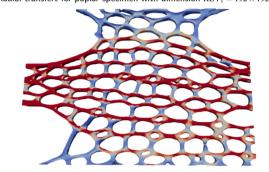
(b) Radial transfert for maple specimen with dimension  $REV_1 = 192 \times 192 \times 6$ .
