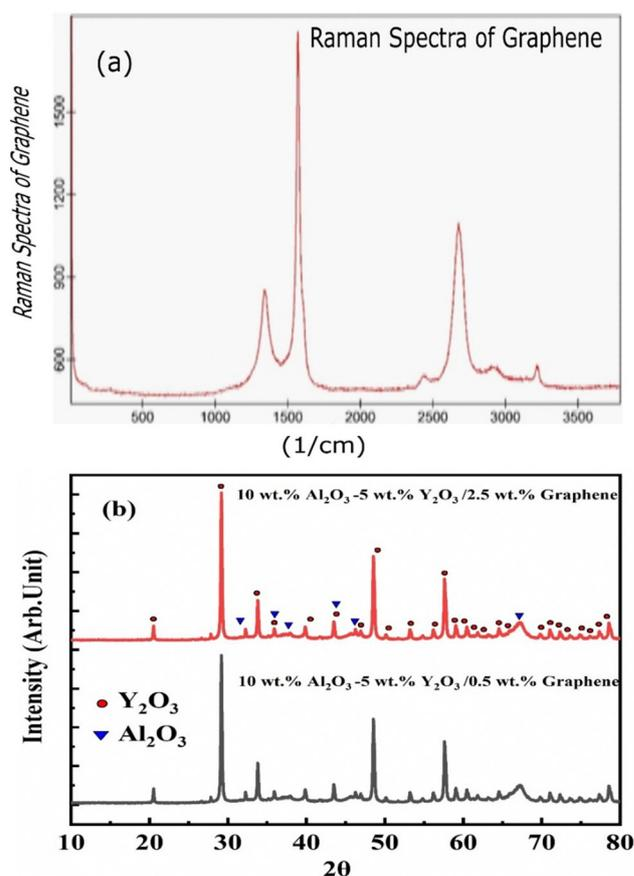
Fig. 4 (a) the Raman spectra of graphene powder, and (b) 10wt% $\text{Al}_2\text{O}_3$ /5wt% $\text{Y}_2\text{O}_3$ /2.5wt%GNSs and 10wt% $\text{Al}_2\text{O}_3$ /5wt% $\text{Y}_2\text{O}_3$ /2.5wt%GNSs nano-composite powders.
