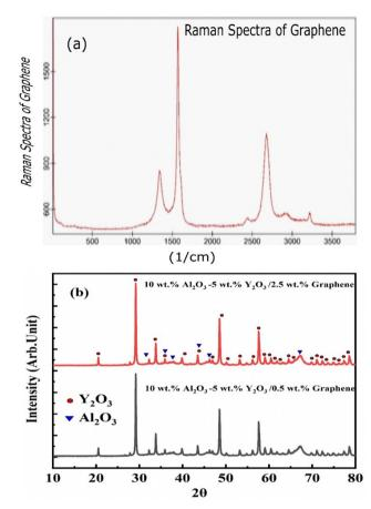
Fig. 4 (a) the Raman spectra of graphene powder, and (b) 10wt%Al<sub>2</sub>O<sub>3</sub>/ 5wt%Y2O3/2.5wt%gGNSs and 10wt%Al2O3/5wt%Y2O3/2.5wt%GNSs nanocomposite powders.
