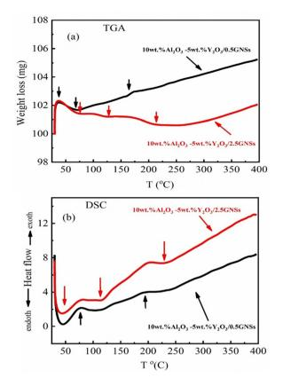
Fig. 5 Thermal analysis (TGA/DSC) of samples with 0.5wt% and 2.5wt% of graphene
