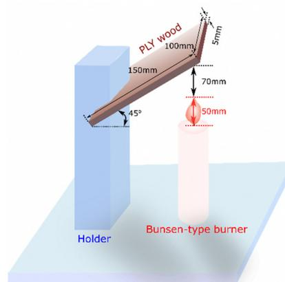
Fig. 1 Fire resistance test system according to Iranian patent no. 67232.<sup>18</sup>
