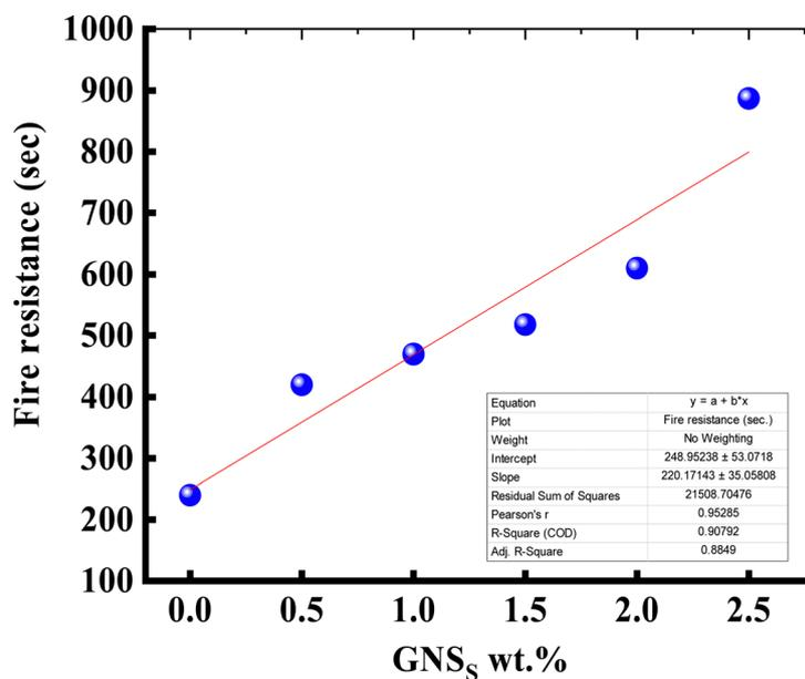
Fig. 8 The effect of GNS content on the fire resistance of wood samples coated with paint with 10wt%Al<sub>2</sub>O<sub>3</sub> and 10wt%Al<sub>2</sub>O<sub>3</sub>/5wt%Y<sub>2</sub>O<sub>3</sub>/xwt%GNSs (x: 0, 0.5, 1.0, 1.5, 2.0, 2.5) mixed powders.
