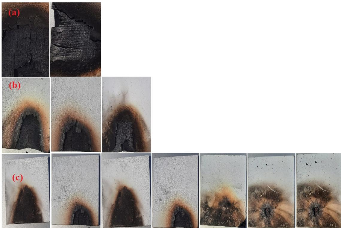
Fig. 7 Wood samples after the fire resistance test: (a) pure wood samples; (b) wood samples treated with paint; (c) wood samples coated with paints of mixed powders: 10wt%Al<sub>2</sub>O<sub>3</sub> and 10wt%Al<sub>2</sub>O<sub>3</sub>/5wt%Y<sub>2</sub>O<sub>3</sub>/xwt%GNSs (x: 0, 0.5, 1.0, 1.5, 2.0, 2.5), respectively.
