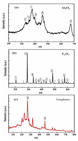
Fig. 3 The XRD test of element powders and mixture powders (a) Al<sub>2</sub>O<sub>3</sub> powder, (b) Y<sub>2</sub>O<sub>3</sub> powder, (c) graphene powder
