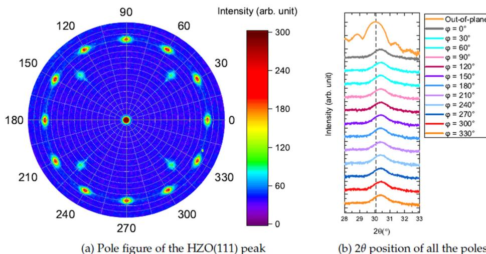
Fig. 4 Panel (a) shows the pole figure of the HZO (111) peak of a 10 nm HZO film on a single crystal STO substrate. The radial angle  $\chi$  ranges from  $0^\circ$  up to  $85^\circ$  and the azimuthal angle  $\phi$  ranges from  $0^\circ$  to  $359^\circ$ . Panel (b) shows the  $2\theta$  position of each pole. The dashed line is drawn at the position of the out-of-plane (111) pole as a guide to the eye.
