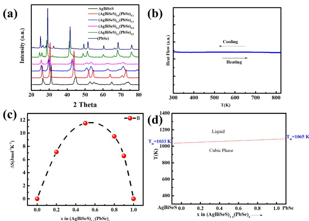
Fig. 1 (a) Room-temperature XRD pattern of  $(\text{AgBiSeS})_{1-x}(\text{PbSe})_x$  ( $x = 0, 0.2, 0.5, 0.8, 0.9, 1.0$ ); (b) DSC curve for the alloy system; (c) calculated configurational entropy vs. composition parameter  $x$  for  $(\text{AgBiSeS})_{1-x}(\text{PbSe})_x$  ( $x = 0, 0.2, 0.5, 0.8, 0.9, 1.0$ ); (d) schematic of temperature-composition plot for the pseudo-binary alloy system depicting stabilized cubic structure in the entire temperature regime.
