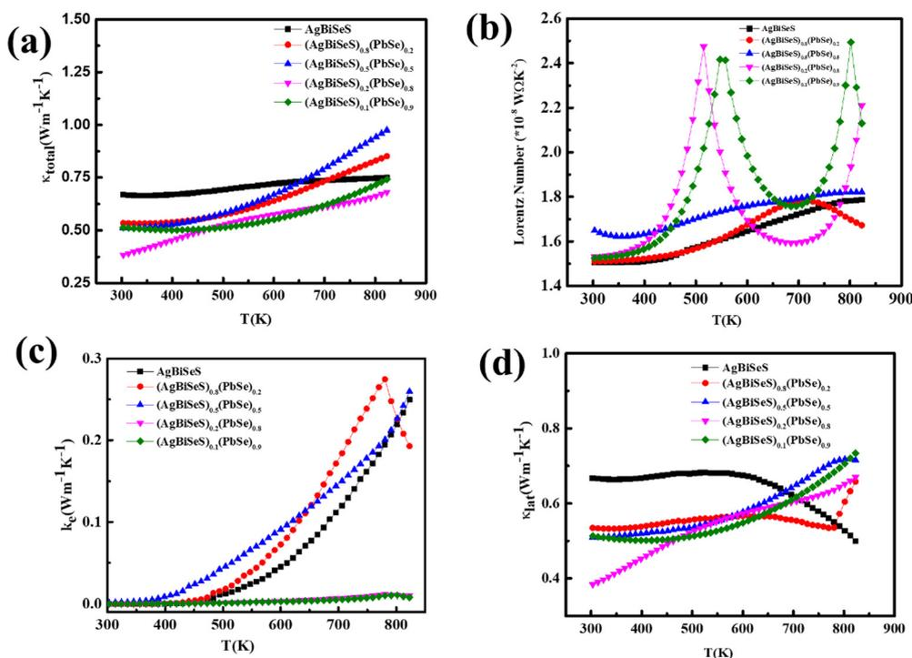
Fig. 6 Temperature-dependent (a) total thermal conductivity; (b) Lorentz number calculated using the Seebeck coeff. values; (c) electronic thermal conductivity; and (c) lattice thermal conductivity of the alloy system  $(\text{AgBiSeS})_{1-x}(\text{PbSe})_x$ .
