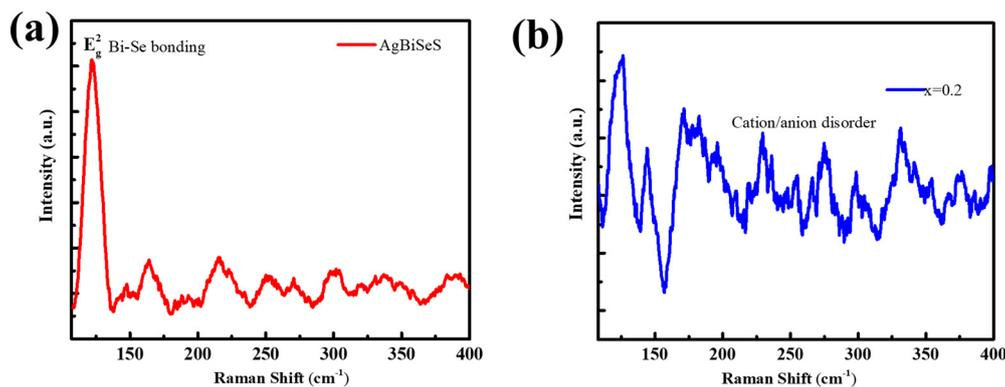
Fig. 2 (a) Room-temperature Raman spectra of AgBiSeS and (AgBiSeS)<sub>0.8</sub>(PbSe)<sub>0.2</sub> illustrating how the increase in the configurational entropy aids in disorder in the system, which eventually evades the Raman peak.
