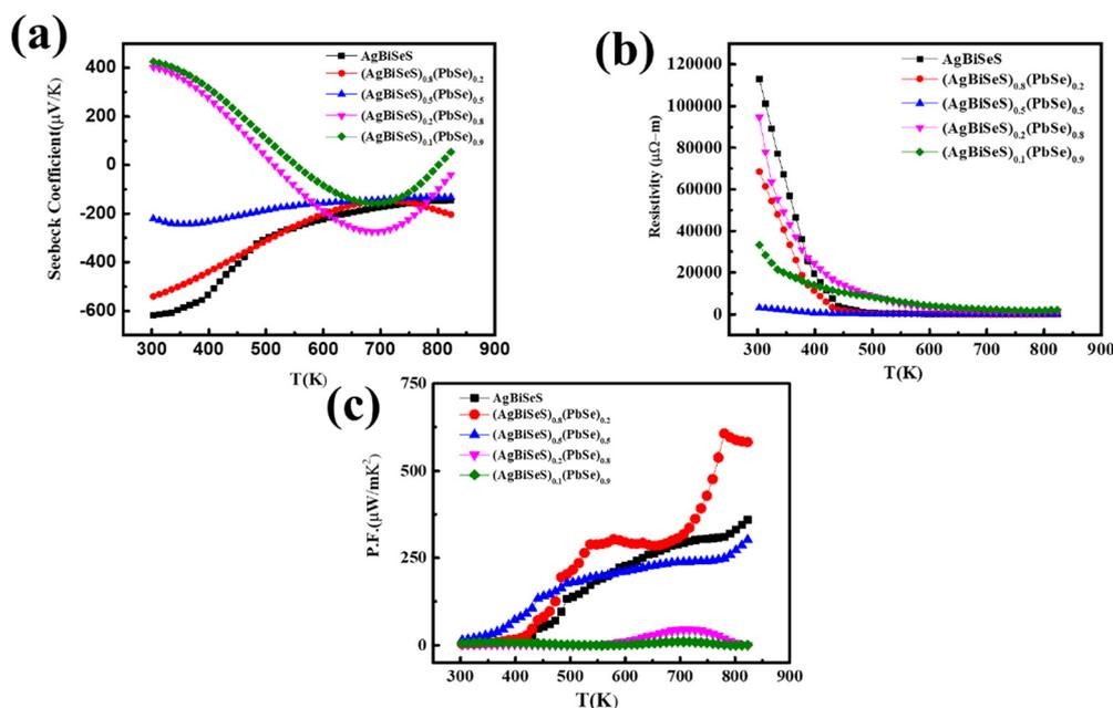
Fig. 4 Temperature-dependent (a) Seebeck coefficient; (b) electrical resistivity and (c) power factor of the alloy system (AgBiSeS)<sub>1-x</sub>(PbSe)<sub>x</sub>.
