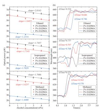
**Fig. 6** Influence of crosslinking density on sensing performance of 2D PHEMA gratings. (a) Sensing sensitivity in the 0–5% concentration range decreased as the crosslinking density of PHEMA increased for each type of alcohol. (b) Response time increased with higher crosslinking density of PHEMA.
