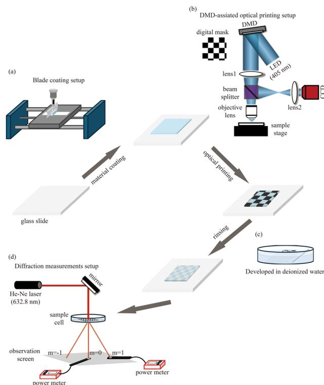
**Fig. 1** Schematic illustration of integration smart materials with DMD-assisted optical printing. (a) Home-built blade coating setup; (b) DMD-assisted optical printing setup; (c) unprocessed material development; (d) optical diffraction efficiency measurement setup.
