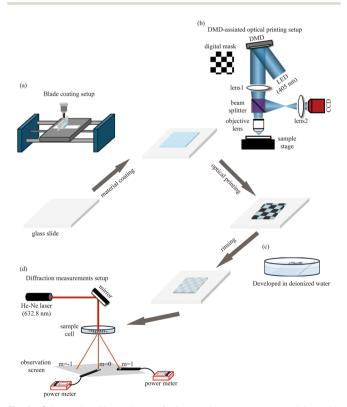
Fig. 1 Schematic illustration of integration smart materials with DMD-assisted optical printing. (a) Home-built blade coating setup; (b) DMD-assisted optical printing setup; (c) unprocessed material developing device; (d) optical diffraction efficiency measurement setup
