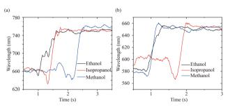
Fig. 5 Time response of printed 1D PHEMA grating (a) and 2D PHEMA grating (b) to different alcohols
