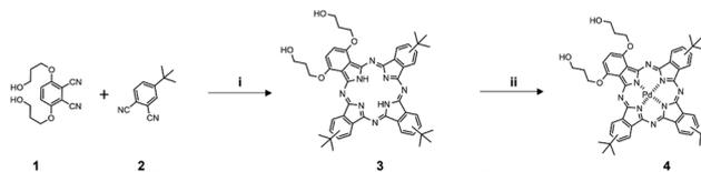
**Scheme 2** Synthetic route to PdBu<sub>3</sub>PROH<sub>2</sub> (4). Reagents and conditions: (i) Li, 1-pentanol, reflux, Ar, 2.5 h; (ii) sodium tetrachloropalladate(II), DMF, reflux, argon, overnight.
