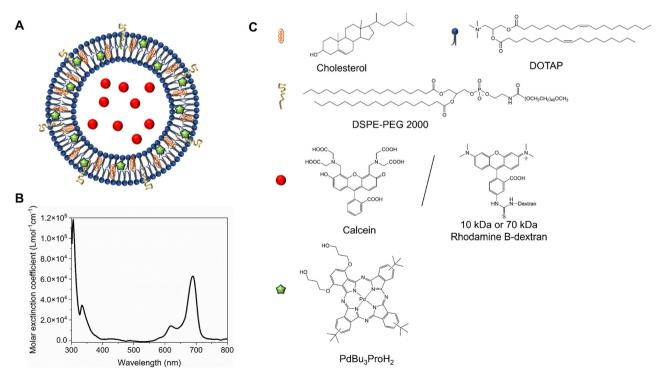
Fig. 1 (A) Structure of liposome, with the following lipid composition DOTAP: Cholesterol: DSPE-PEG 2000 in ratio 45:50:5. (B) Absorption spectrum of PdBu<sub>3</sub>PrOH<sub>2</sub> in Pyridine: H<sub>2</sub>O 3:1 (v/v). Chemical structure of cholesterol, DSPE-PEG 2000, Calcein, rhodamine B dextran, and PdBu<sub>3</sub>PrOH<sub>2</sub>.
