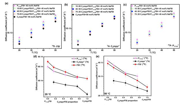
Fig. 3 Diffusion coefficients of (a) anion ( $^{19}$ F), (b)  $C_3$ mpyr cation ( $^{11}$ H), (c)  $P_{111i4}$  cation ( $^{31}$ P) as a function of  $C_3$ mpyrFSI proportion, (d) diffusion coefficients at 20 °C (e) at 50 °C.
