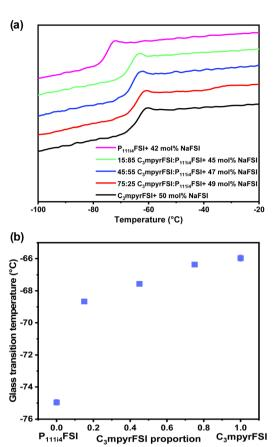
Fig. 1 (a) DSC heating traces of the mixed P<sub>111i4</sub>FSI and C<sub>3</sub>mpyrFSI with a saturated NaFSI system. (b) Glass transition temperature as a function of C<sub>3</sub>mpyrFSI proportion.
