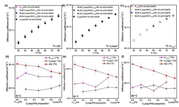
Fig. 7 Diffusion coefficient of (a) anion ( $^{19}$ F), (b)  $C_3$ mpyr cations ( $^{11}$ H), (c)  $P_{111i4}$  cations ( $^{31}$ P) as a function of  $C_3$ mpyrFSI proportion, (d) diffusion coefficients at 20 °C (e) at 50 °C (f) at 80 °C.
