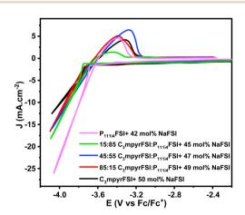
Fig. 4 Cyclic voltammetry curves for the mixed  $P_{11114}FSI$  and  $C_3mpyrFSI$  with a saturated NaFSI system during the 1st cycle.
