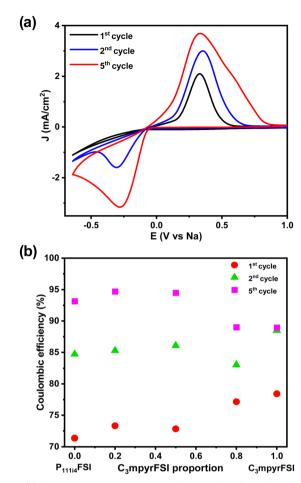
Fig. 9 (a) Cyclic voltammetry curves for C<sub>3</sub>mpyrFSI + 42 mol% NaFSI from 1st, 2nd and 5th cycle. (b) Coulombic efficiencies as a function of C<sub>3</sub>mpyrFSI proportion.
