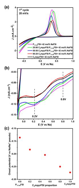
Fig. 8 (a) Cyclic voltammetry curves for the mixed P<sub>111i4</sub>FSI and C<sub>3</sub>mpyrFSI with 42 mol% NaFSI system at 1st cycle, (b) the enlarged reduction process, and (c) the onset potential as a function of C<sub>3</sub>mpyrFSI proportion.
