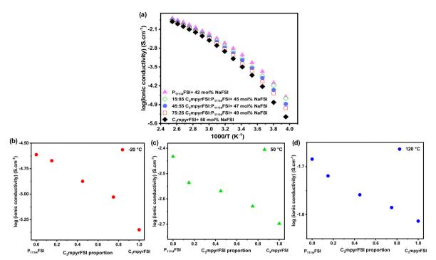
Fig. 2 (a) Temperature-dependent ionic conductivity, (b) the ionic conductivity at -20 °C, (c) the ionic conductivity at 50 °C, (d) the ionic conductivity at 120 °C.
