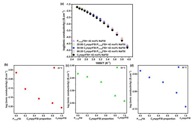
Fig. 6 (a) Temperature-dependent ionic conductivity of the mixed P<sub>11114</sub>FSI and C<sub>3</sub>mpyrFSI with 42 mol% NaFSI system, (b) the ionic conductivity at 20 °C, (c) the ionic conductivity at 50 °C, (d) the ionic conductivity at 80 °C.
