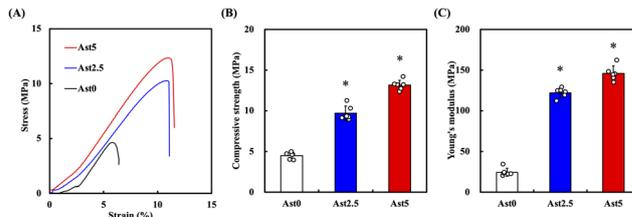
Fig. 3 Mechanical stress analysis of AstCS scaffolds. (A) Stress–strain curve. (B) compressive strength and (C) Young's modulus of Ast0, Ast2, and Ast5 scaffolds. Data presented are  $n = 6$  for each group.
