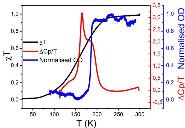
Fig. 10 Thermal-dependence of the contribution HS fraction of sample **1** undergoing the spin transition derived from magnetic data (black curve) and OM technique (blue curve), plotted with DSC measurements (red curve), showing excellent agreement.
