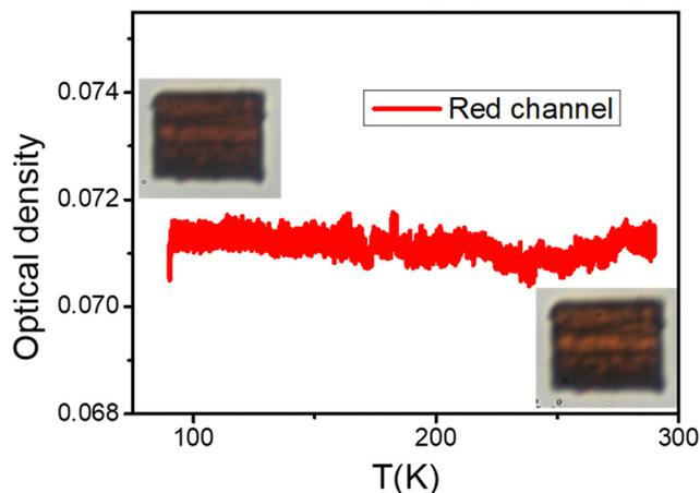
Fig. 9 Thermal-dependence of the OD, derived from the red channel, of a single crystal of compound **1**, studied under vacuum, showing the absence of the colour change. Insets: two typical images of the crystal at 90 K (top left) and at 290 K (bottom right).
