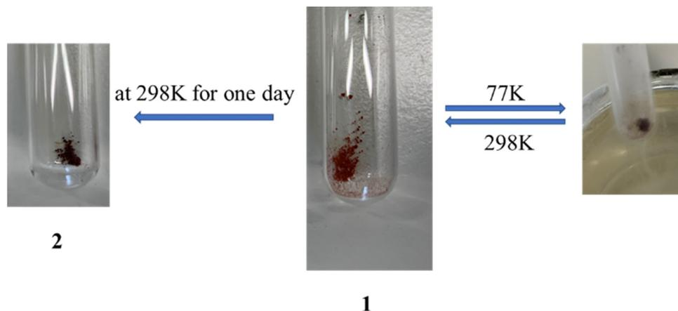
Fig. 1 Colour changes of **1** at 77 K and 298 K, as well as after one day at r.t. leading to **2**.
