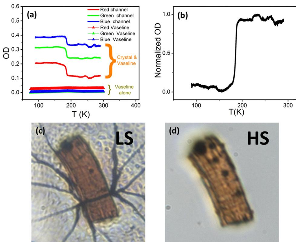
Fig. 8 (a) OD measurements derived from the three-colour channels (RGB) as a function of temperature on a single crystal of **1** of size,  $138 \times 46 \mu\text{m}^2$ , protected by Vaseline and OD measurements (RGB) of Vaseline alone in triangles. (b) Normalized value of the OD as a function of temperature derived from panel (a) (green channel), which is proportional to the HS fraction ( $n_{\text{HS}}$ ). Images of the crystal at 90 K (c) and 290 K (d), respectively.
