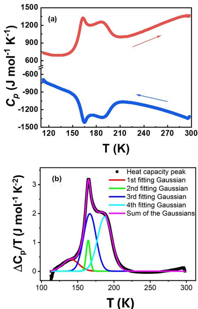
Fig. 7 (a) Heat capacity thermal profile in cooling and warming modes of **1** recorded at a scan rate of  $2 \text{ K min}^{-1}$ . (b) Gaussian fitting of the heat capacity excess vs. temperature, derived from panel (a) along the heating process, considering four contributions.
