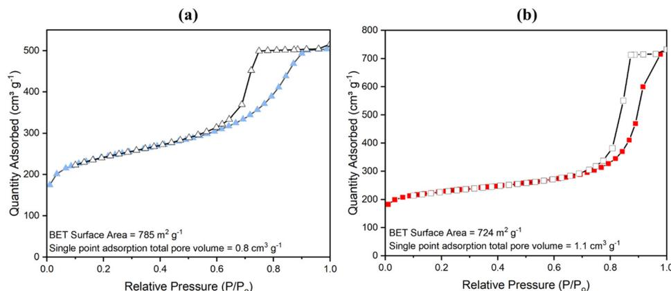
Fig. 4 N<sub>2</sub> gas adsorption isotherms measured at 77 K for (a)  $\text{monoUiO-66-NH}_2\text{-30\%-B}$  (solid triangles represent adsorption, and open triangles denote desorption); (b)  $\text{monoUiO-66-NH}_2\text{-30\%-A}$  (solid squares represent adsorption, and open squares denote desorption).
