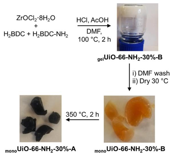
**Scheme 1** Synthesis of monoUiO-66-NH<sub>2</sub>-30%-B (orange) and monoUiO-66-NH<sub>2</sub>-30%-A (black) from gelUiO-66-NH<sub>2</sub>-30%-B. H<sub>2</sub>BDC-NH<sub>2</sub> used was 30% by weight with respect to H<sub>2</sub>BDC.
