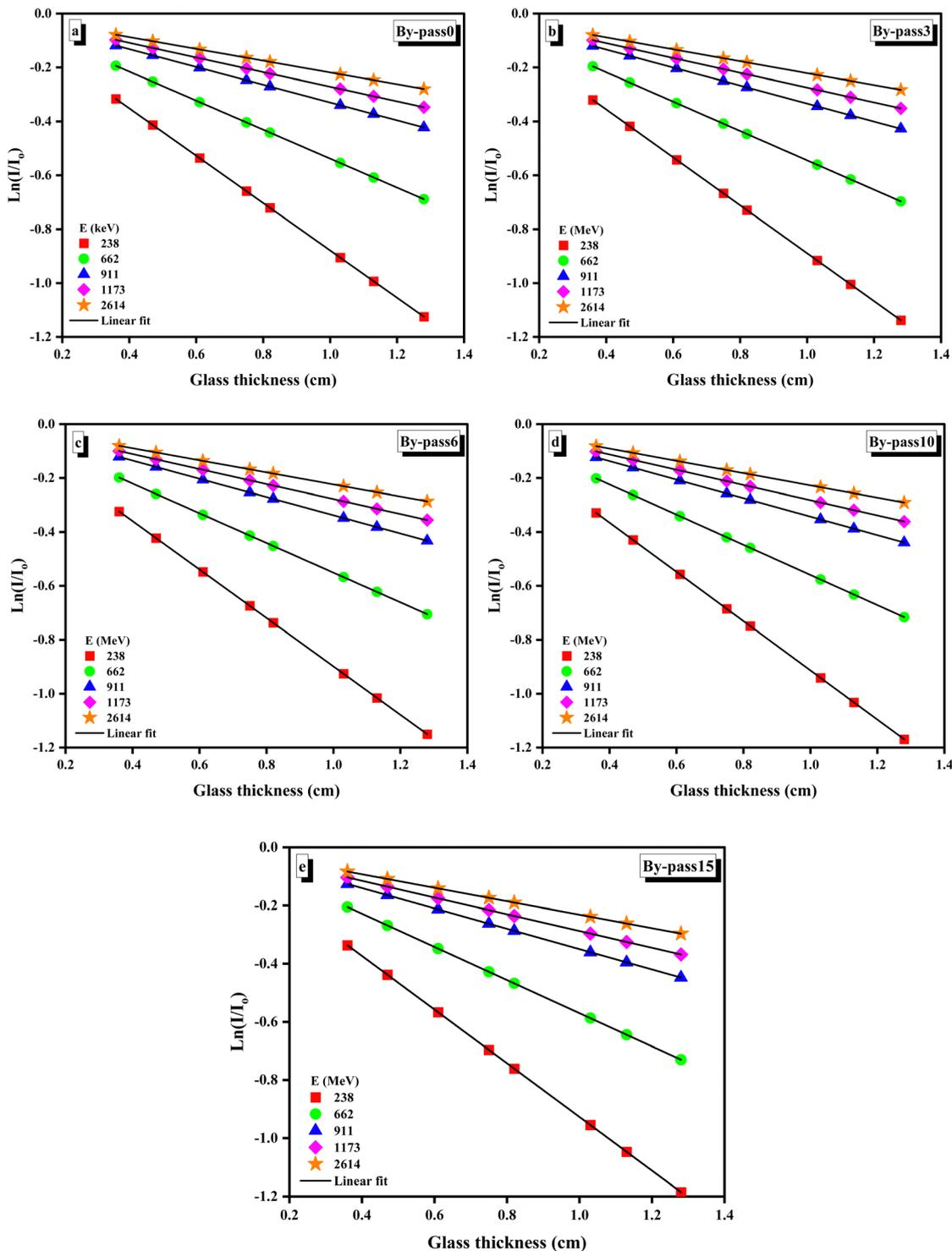
Fig. 9 (a)–(e) Transmission factor ( $\ln(I/I_0)$ ) against glass thickness at a selected photon energy.
