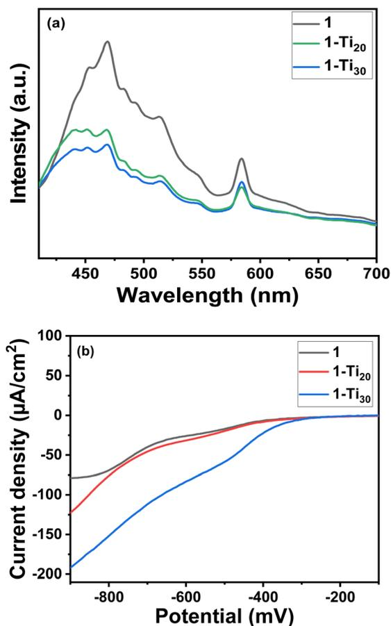
Fig. 4 (a) Photoluminescent spectra of the MOFs at an excitation wavelength of 395 nm. (b) Photocurrent experiment showing current produced for different MOFs in the light on condition.
