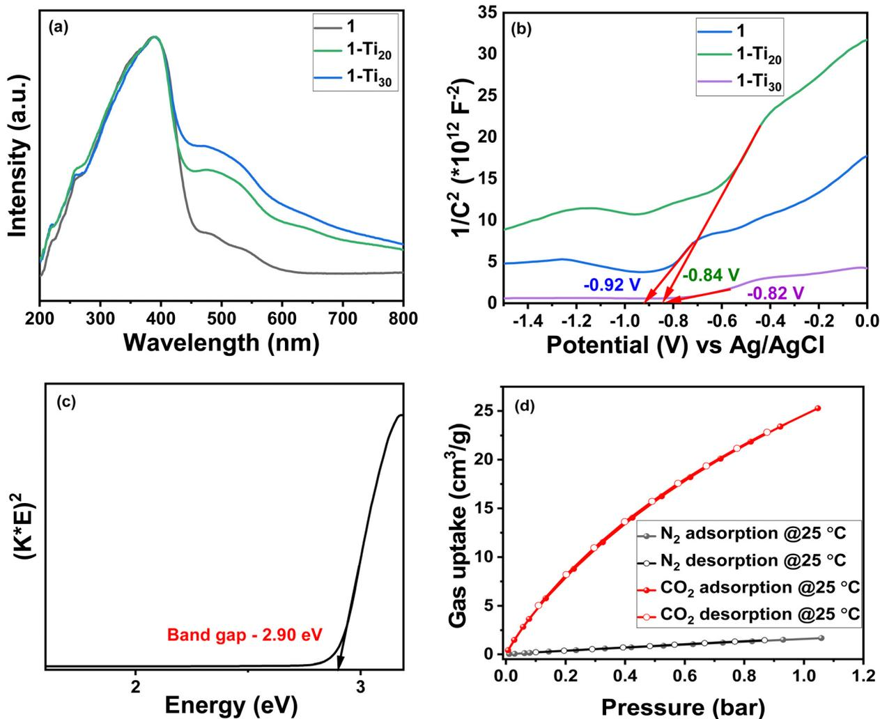
Fig. 2 (a) UV-vis absorption spectra of **1**, **1-Ti<sub>20</sub>**, and **1-Ti<sub>30</sub>** showing major absorption peak broadening at 388 nm and secondary peak broadening at 510 nm for Ti-exchanged samples. (b) Mott-Schottky plot for the conduction band position determination at a 500 Hz frequency. (c) Kubelka-Munk plot showing the band gap of **1**. (d) CO<sub>2</sub> and N<sub>2</sub> adsorption isotherms for **1**.
