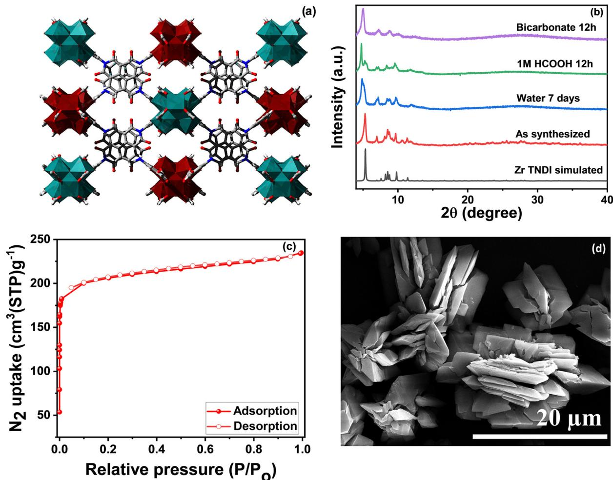
Fig. 1 (a) Packing diagram of the 2-fold interpenetrated structure of the Zr-TNDI MOF (**1**). Zr, C, N, and O atoms are shown in maroon/light blue, grey, blue, and red colors, respectively.<sup>21</sup> (b) PXRD of **1** showing its bulk purity and stability in water, 1 M formic acid, and 0.1 M bicarbonate solution. (c) BET surface area measurement and (d) SEM image of **1** showing an intergrown rod-shaped morphology.
