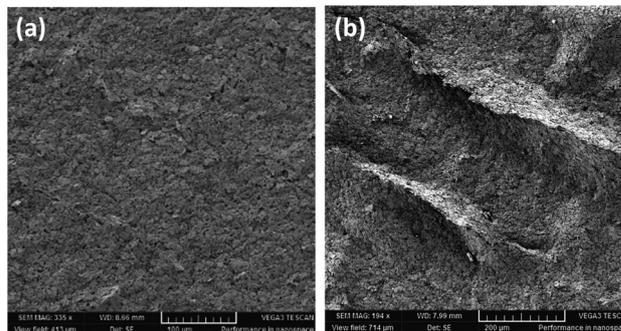
Fig. 6 SEM images for screen printed pattern investigation: (a) an unstretched sample and (b) a stretched-then-relaxed sample.
