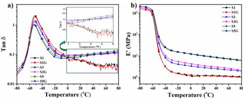
Fig. 8 DMA temperature sweep plot – (a)  $\tan \delta vs$ . temperature plot and (b) storage modulus vs. temperature plot of the NR vulcanizates.
