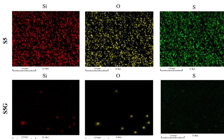
Fig. 15 FIB-SEM images of the 50 phr silica filled NR vulcanizate (S5) and the 50 phr silica–5 phr glucose filled NR vulcanizate (S5G).
