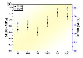
(a) Hardness and (b) modulus plots of the NR vulcanizates.
