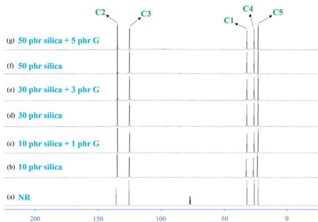
Fig. 9 (a) The solution-state  $^{13}\text{C}$  NMR spectrum of unvulcanized NR and the rubber-state  $^{13}\text{C}$  NMR spectra of the vulcanized natural rubbers prepared with silica and with silica and glucose. (b) 10 phr silica, (c) 10 phr silica with 1 phr glucose, (d) 30 phr silica, (e) 30 phr silica with 3 phr glucose, (f) 50 phr silica, and (g) 50 phr silica with 5 phr glucose, together with the solution-state  $^{13}\text{C}$  NMR spectrum of unvulcanized natural rubber.
