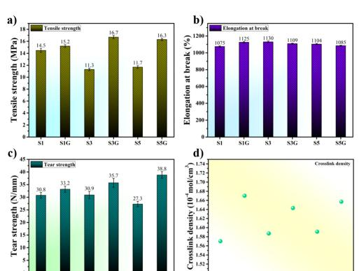
S3G Fig. 6 (a) Tensile, (b) elongation, (c) tear strength, and (d) crosslink density plots of the NR vulcanizates
