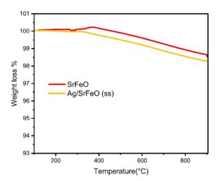
Fig. 3  $\,$  TGA of the support SrFeO $_3$  and catalyst Ag/SrFeO $_3$  from room temperature to 950  $^{\circ}$ C in air.
