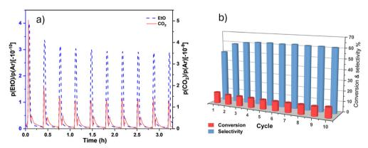
Fig. 9 Used catalyst performance. The signal intensity and stability (a) of CO2 and EtO as a function of reaction time and (b) selectivity towards EtO and conversion of C<sub>2</sub>H<sub>4</sub> were obtained from 10 epoxidation cycles.
