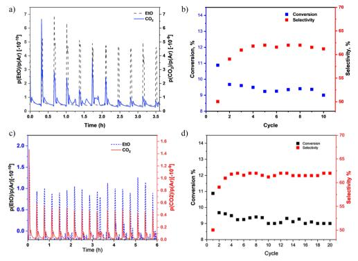
Fig. 8 Fresh catalyst performance. The signal intensity and stability (a) of CO<sub>2</sub> and EO as a function of reaction time from 10 epoxidation cycles, (b) selectivity towards EO and conversion of C<sub>2</sub>H<sub>4</sub> obtained from 10 epoxidation cycles, (c) signal intensity and stability of CO<sub>2</sub> and EtO as a function of reaction time from 20 epoxidation cycles and (d) selectivity towards EtO and conversion of C<sub>2</sub>H<sub>4</sub> obtained from 20 epoxidation cycles.
