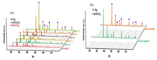
Fig. 4 (a) X-ray diffraction patterns of the solid-state synthesized AgSrFeO<sub>3</sub> calcined at various temperatures between 500  $^{\circ}$ C and 900  $^{\circ}$ C (control is fresh AgSrFeO<sub>3</sub>) (b) comparison between the fresh catalyst and the spent catalyst.
