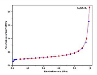
Fig. 6 Nitrogen adsorption-desorption isotherms of AgSrFeO<sub>3</sub> from ball milling.
