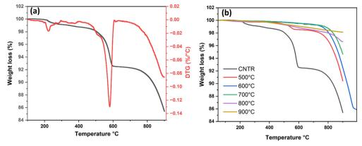
Fig. 2 (a) TGA-analysis curve for the fresh Ag/SrFeO<sub>3</sub> catalyst, (b) TGA curve of the Ag/SrFeO<sub>3</sub> catalyst calcined at different temperatures.
