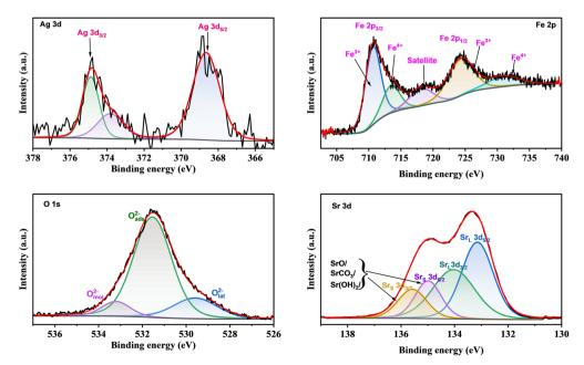
Fig. 7 Fitted XPS spectra of Ag 3d, Fe 2p, O 1s and Sr 3d of the Ag/SrFeO<sub>3</sub>(ss) fresh catalyst.
