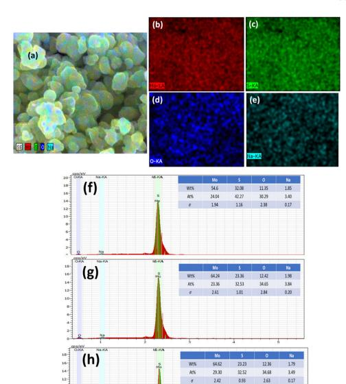
Fig. 4 Elemental mapping. (a) FESEM image of the 0-MoS<sub>2</sub> sample, (b) molybdenum element in red, (c) sulphur element in green, (d) oxygen in blue, and (e) sodium in light blue. Energy dispersive X-ray spectroscopy (EDS) study of (f) 0-MoS<sub>2</sub>, (g) 2-MoS<sub>2</sub>, and (h) 4-MoS<sub>2</sub> samples.
