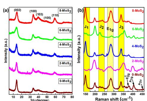
Fig. 2 (a) Corresponds to the X-ray diffraction pattern and (b) Raman spectra of the prepared MoS<sub>2</sub> samples with duration time of 0, 2, 4, 6, and 8 days.
