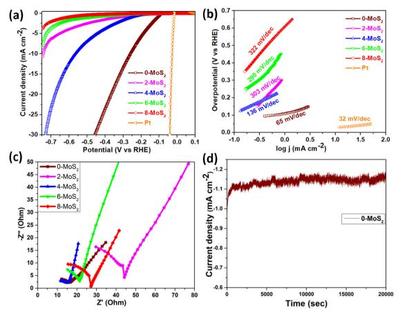
Fig. 6 Electrocatalytic performance of Pt- and MoS<sub>2</sub>-based material. (a) Linear sweep voltammetry (LSV) curve, (b) Tafel slope, (c) electrochemical impedance spectroscopy (EIS) of 0-MoS2, 2-MoS2, 4-MoS2, 6-MoS2, and 8-MoS2, and (d) stability test of 0-MoS2.
