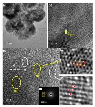
Fig. 5 (a) Transmission electron microscopy image, (b) high-resolution transmission electron microscopy (HRTEM) image of 0-MoS<sub>2</sub>, (c) low magnification HRTEM of 1T/2H-MoS<sub>2</sub>, (d) HRTEM image of region magnified by the yellow ellipse in (a) and (e) white region magnified in (a) and (f) selected area electron diffraction pattern of 0-MoS<sub>2</sub>.
