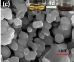
Fig. 3 FESEM images of (a) 0-MoS<sub>2</sub>, (b) after 2 days, and (c) after 4 days. The inset shows solution colour changes as time increased from 0 to 4 days
