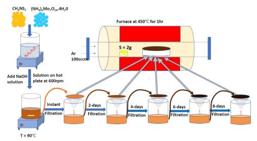
Fig. 1 Schematic representation of the experimental setup: A wet chemical method was used to prepare MoS<sub>2</sub> material by varying the duration time. Further annealing was conducted under a sulfur atmosphere at 450 °C for 1 hour.
