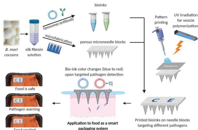
Fig. 6 A schematic illustration of the fabrication of BI-SF-MNs and their application. The image was reproduced with permission<sup>89</sup> from Wiley, copyright@2021.
