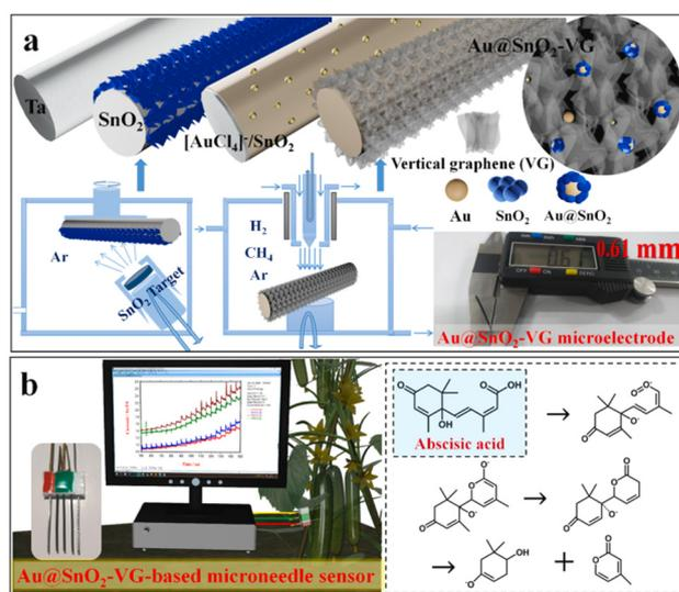
Fig. 3 A schematic illustration of the (a) fabrication of Au-SnO<sub>2</sub>-VG-MN, and (b) detection mechanism of ABA. The image was reproduced with permission<sup>62</sup> from Elsevier, copyright@2021.
