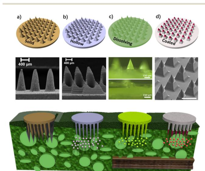
Fig. 2 Types of MNs and their application in agriculture: (a) solid, (b) hollow, (c) dissolving, and (d) coated-MNs. The image was reproduced with permission<sup>40</sup> from Elsevier, copyright@2023.
