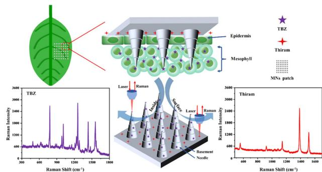
Fig. 5 A schematic representation of the pesticide residue in agricultural products using MNs. The image was reproduced with permission<sup>86</sup> from ACS, copyright@2023.
