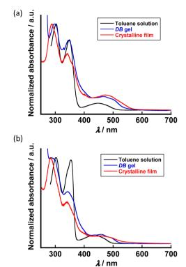
Fig. 4 UV-Vis spectra of (a) FL-1 and (b) FL-2 in the toluene solution (10 µM), dodecylbenzene gel and crystalline film states
