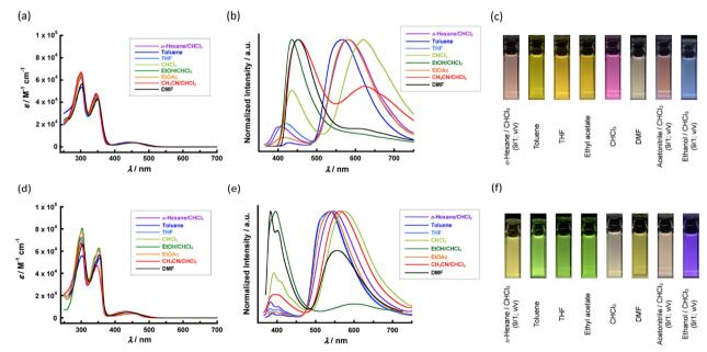
Fig. 5 (a) and (d) UV-Vis spectra of (a) FL-1 and (d) FL-2 in solutions diluted by the various solvents (10 μM). (b) and (e) PL spectra of (b) FL-1 and (e) FL-2 in solutions diluted by various solvents (10  $\mu$ M). (c) and (f) Photographs for various solutions (10  $\mu$ M) of (c) **FL-1** and (f) **FL-2** in vials under the UV-light (355 nm) irradiation
