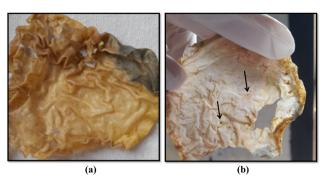
Fig. 10 Signs of biodegradation [(a) color changes and darkening of the film. (b) Formation of multiple holes in the film, a sign of bulk-erosion-type degradation].
