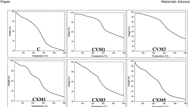
Fig. 6 Thermal analysis (C: pristine chitosan, CVM1: chitosan-vanillin composite with 1% reinforced MMT, CVM3: chitosan-vanillin composite with 3% reinforced MMT CXM1: chitosan-xanthan gum composite with 1% reinforced MMT, CXM3: chitosan-xanthan gum composite with 3% reinforced MMT, CXM5: chitosan-xanthan gum composite with 5% reinforced MMT)
