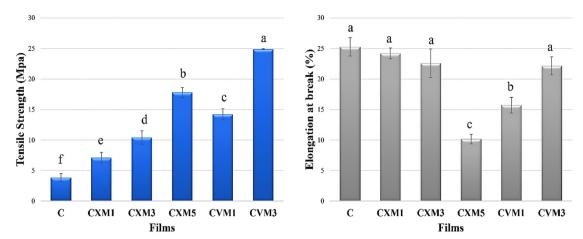
Fig. 5 Mechanical capabilities of all the manufactured films [different letters represent significantly different values at  $(p \le 0.05)$  using Tukey's test (mean ± standard deviation, n = 3)] (C = pristine chitosan film, CXM1 = chitosan-xanthan qum blend with 1% MMT, CXM3 = chitosan-xanthan qum blend with 3% MMT, CXM5 = chitosan-xanthan gum blend with 5% MMT, CVM1 = chitosan-vanillin blend with 1% MMT, and CVM3 = chitosan-vanillin blend with 1% MMT)
