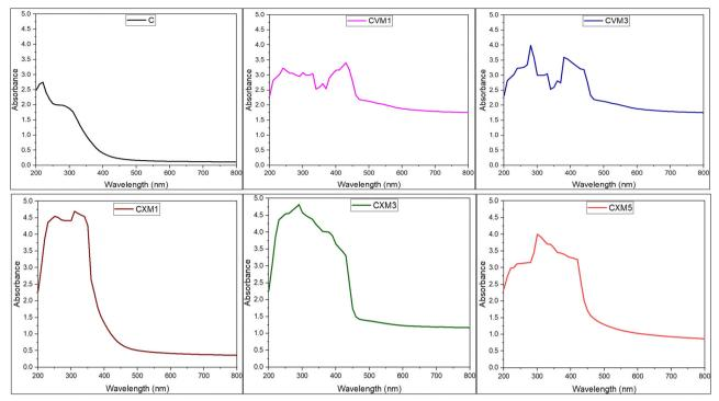
Fig. 8 UV-blocking capacity of all the manufactured films (C: pristine chitosan, CVM1: chitosan-vanillin composite with 1% reinforced MMT, CVM3: chitosan-vanillin composite with 3% reinforced MMT CXM1: chitosan-xanthan gum composite with 1% reinforced MMT, CXM3: chitosan-xanthan gum composite with 3% reinforced MMT, and CXM5: chitosan-xanthan gum composite with 5% reinforced MMT).
