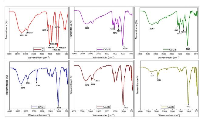
Fig. 4 FTIR spectra of all the fabricated films (C: pristine chitosan, CVM1: chitosan, vanillin composite with 1% reinforced MMT, CVM3: chitosan, vanillin composite with 3% reinforced MMT CXM1: chitosan-xanthan gum composite with 1% reinforced MMT, CXM3: chitosan-xanthan gum composite with 3% reinforced MMT, CXM5: chitosan-xanthan gum composite with 5% reinforced MMT)
