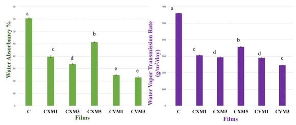
Fig. 9 Water absorbency and water vapor transmission rate of all the synthesized films [different letters within a column represent significantly different values at ( $p \le 0.05$ ) using Tukey's test (mean  $\pm$  standard deviation, n = 3)].
