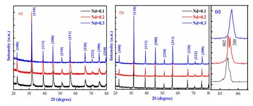
Fig. 1 X-ray diffraction patterns of the  $(Ba_{1-x}Nd_x)(Ti0_8Co_{0.2})O_3$  samples (x = 0.10, 0.20 and 0.30 mol%) (a) calcined powder at  $1200 \, ^{\circ}C/3 \, h$ , (b) sintered ceramics at 1375 °C/3 h and (c) effect of Nd doping in the Nd<sub>x</sub>Ba<sub>1-x</sub>Ti<sub>0.8</sub>Co<sub>0.2</sub>O<sub>3</sub> composite.
