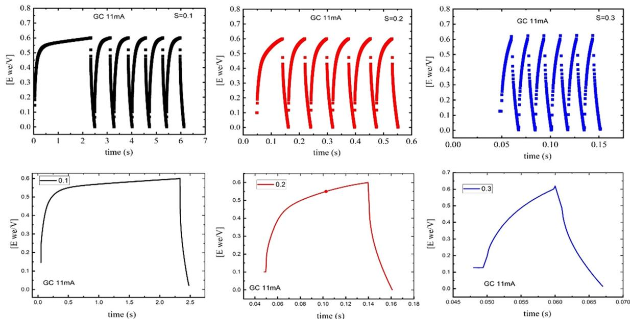
Fig. 7 The charge/discharge curves of  $\text{Nd}_x\text{Ba}_{1-x}\text{Ti}_{0.8}\text{Co}_{0.2}\text{O}_3$ , where  $x = 0.10, 0.20$  &  $0.30$  mol% supercapacitor at constant currents.
