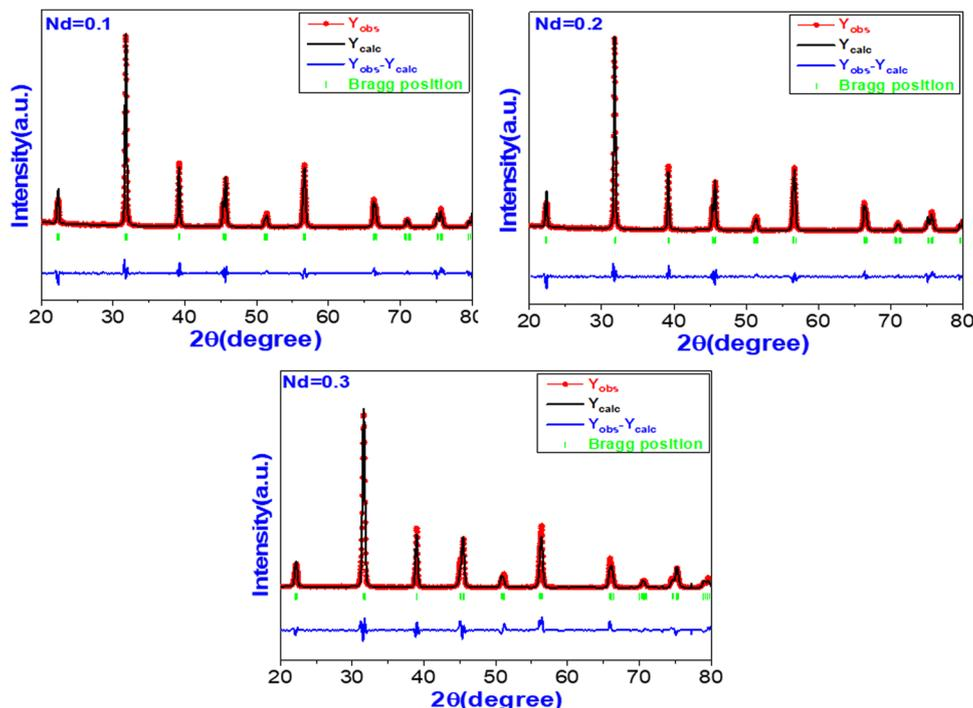
Fig. 2 Rietveld-refined XRD patterns of BNTC sintered ceramics.
