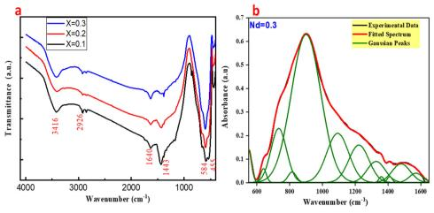
(a) FT-IR spectra of BN<sub>x</sub>TC samples (x = 0.10, 0.20 and 0.30 mol%); (b) deconvolution process for the IR spectrum for Nd = 0.3 calcined powder.
