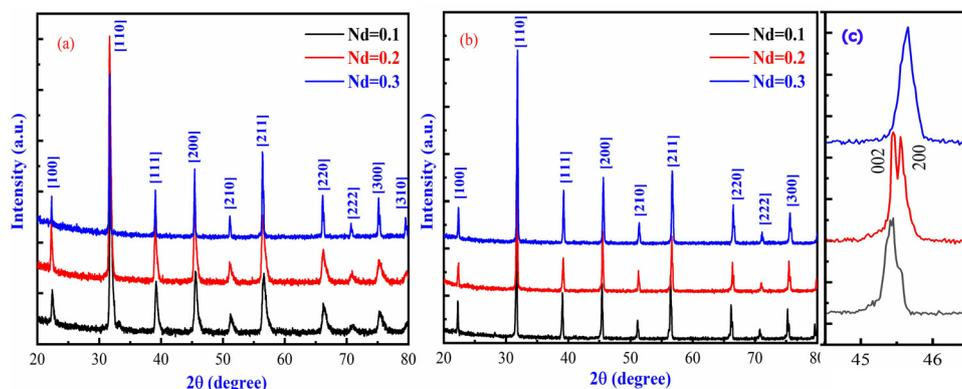
Fig. 1 X-ray diffraction patterns of the  $(\text{Ba}_{1-x}\text{Nd}_x)(\text{Ti}_{0.8}\text{Co}_{0.2})\text{O}_3$  samples ( $x = 0.10, 0.20$  and  $0.30$  mol%) (a) calcined powder at 1200  $^{\circ}\text{C}$ /3 h, (b) sintered ceramics at 1375  $^{\circ}\text{C}$ /3 h and (c) effect of Nd doping in the  $\text{Nd}_x\text{Ba}_{1-x}\text{Ti}_{0.8}\text{Co}_{0.2}\text{O}_3$  composite.
