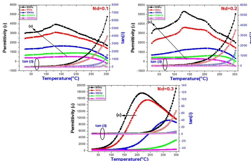
Fig. 4 Temperature dependence dielectric constant ( $\epsilon_r$ ) and dielectric tangent loss,  $\tan(\delta)$  of  $(\text{Ba}_{1-x}\text{Nd}_x)(\text{Ti}_{0.8}\text{Co}_{0.2})\text{O}_3$  composites ( $x = 0.10, 0.20$  and  $0.30$  mol%).
