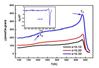
Fig. 5 Temperature dependence susceptibility of (Ba<sub>1-x</sub>Nd<sub>x</sub>)(Ti<sub>0.8</sub>Co<sub>0.2</sub>)O<sub>3</sub> (x = 0.10, 0.20 and 0.30 mol%)
