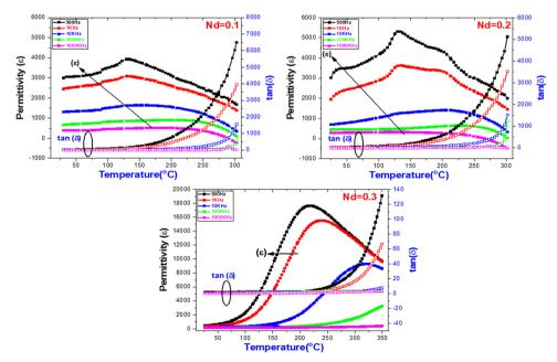
Fig. 4 Temperature dependence dielectric constant ( $\varepsilon_r$ ) and dielectric tangent loss,  $\tan{(\delta)}$  of  $(Ba_{1-x}Nd_x)(Ti_{0.8}Co_{0.2})O_3$  composites (x = 0.10, 0.20 and 0.30 mol%).
