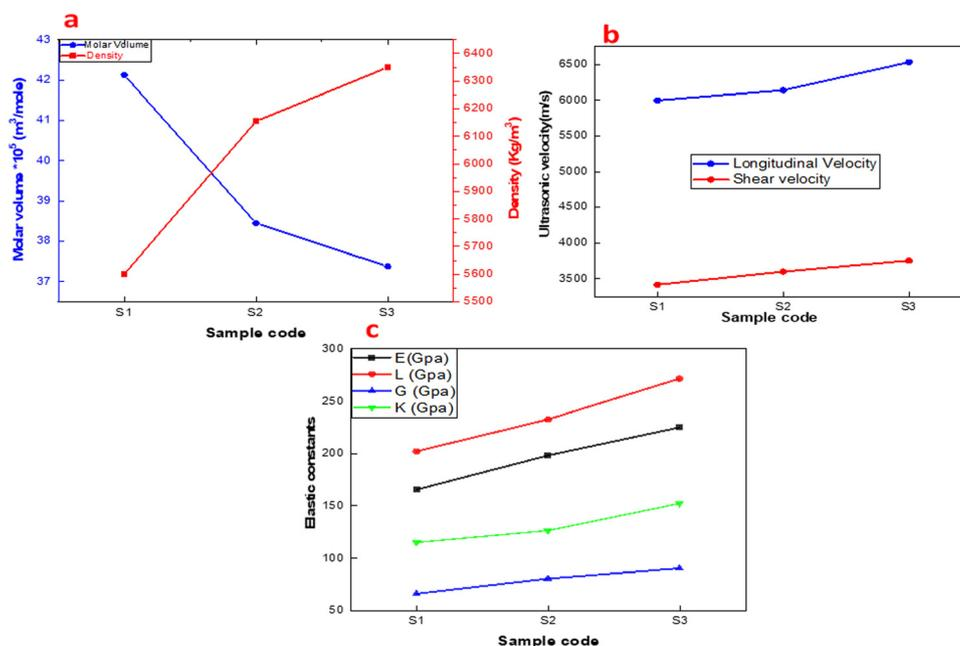
**Fig. 6** (a) Molar volume and density (b) Longitudinal and shear velocities and (c) elastic modulus of (Ba<sub>1-x</sub>Nd<sub>x</sub>)(Ti<sub>0.8</sub>Co<sub>0.2</sub>)O<sub>3</sub> composites ( $x = 0.10, 0.20$  and  $0.30$  mol%).
