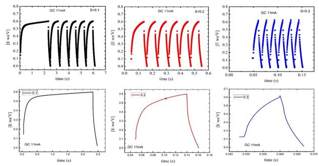
The charge/discharge curves of  $Nd_xBa_{1-x}Ti_{0.8}Co_{0.2}O_3$ , where x = 0.10, 0.20 & 0.30 mol% supercapacitor at constant currents.
