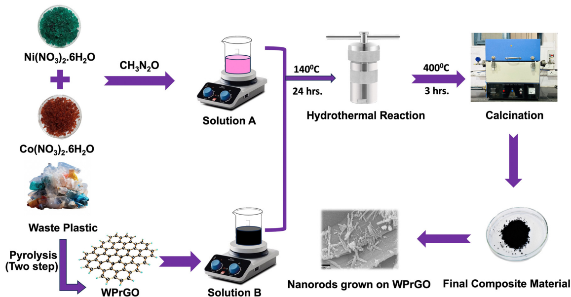
Fig. 1 Schematic representation of the synthesis of the NiCo 2 O 4 @WPrGO composite material.
