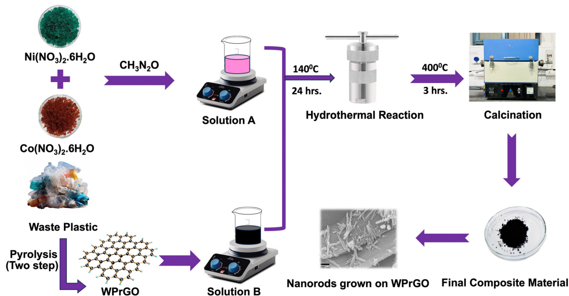
Fig. 1 Schematic representation of the synthesis of the \text{NiCo}_2\text{O}_4/\text{WPrGO} composite material.
