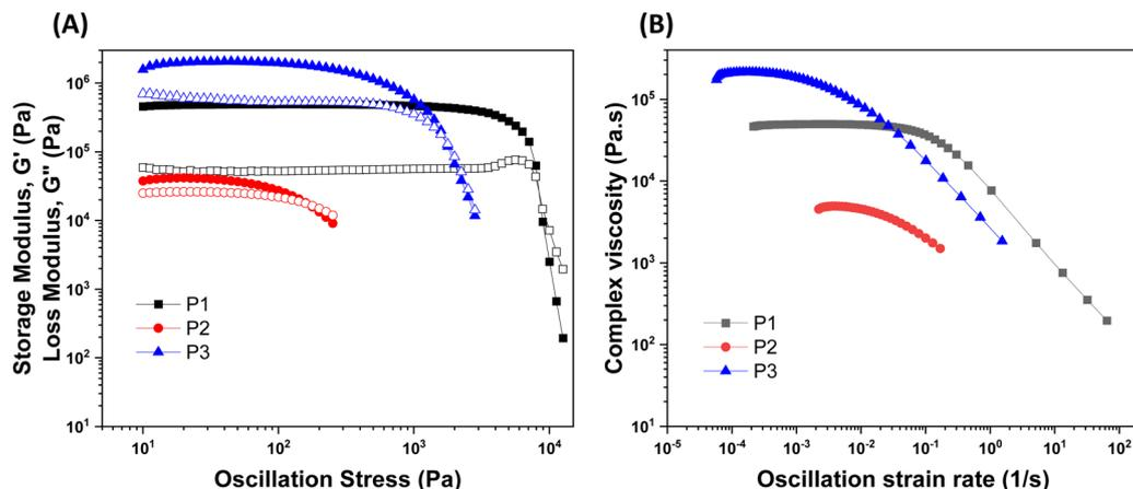
Fig. 2 (A) Storage ( $G'$ , filled symbols) and loss ( $G''$ , unfilled symbols) moduli as a function of oscillation stress and (B) complex viscosity as a function of oscillation strain rate for the P1, P2, and P3 resins.
