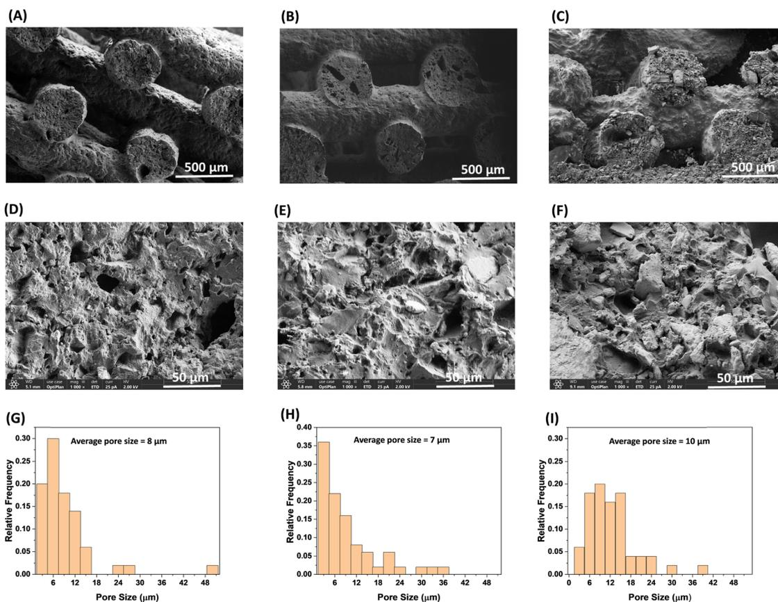
**Fig. 4** SEM images (A)–(F) at different magnification of cross-section and pore size distribution (D)–(F) of printed samples after extraction of NaCl. ((A), (D) and (G) for sample P1, (B), (E), and (H) for sample P2, and (C), (F), and (I) for sample P3).
