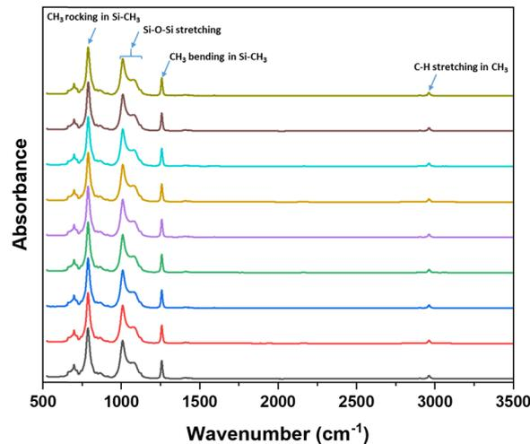
Fig. 1 FT-IR spectra of the ground resins taken at different time intervals.
