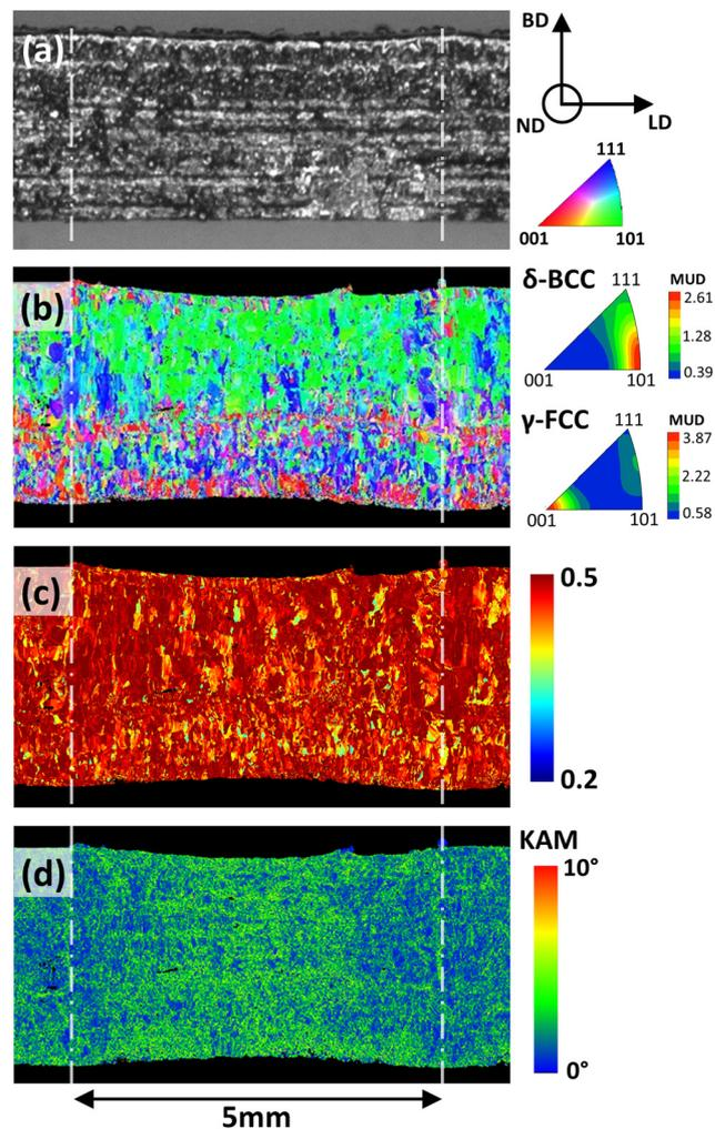
Fig. 18 Periodic necking in the as-built  $45^\circ$  sample: (a) optical micrograph of sample surface showing spatial necking along sample thickness, (b) crystallographic texture map in the normal direction (ND) and corresponding inverse pole figures, (c) Schmid factor map and (d) KAM map.
