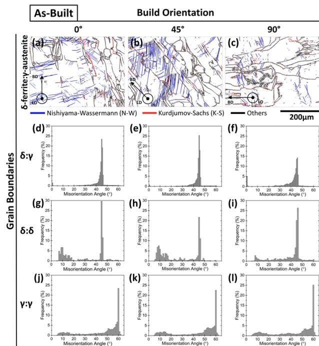
Fig. 11 As-built samples: (a)–(c) orientation relationships of  $\delta$ -ferrite: $\gamma$ -austenite interfaces; (b) misorientation angle histograms for the (d)–(f)  $\delta$ -ferrite: $\gamma$ -austenite, (g)–(i)  $\delta$ -ferrite: $\delta$ -ferrite and (j)–(l)  $\gamma$ -austenite: $\gamma$ -austenite grain boundaries at each build orientation.
