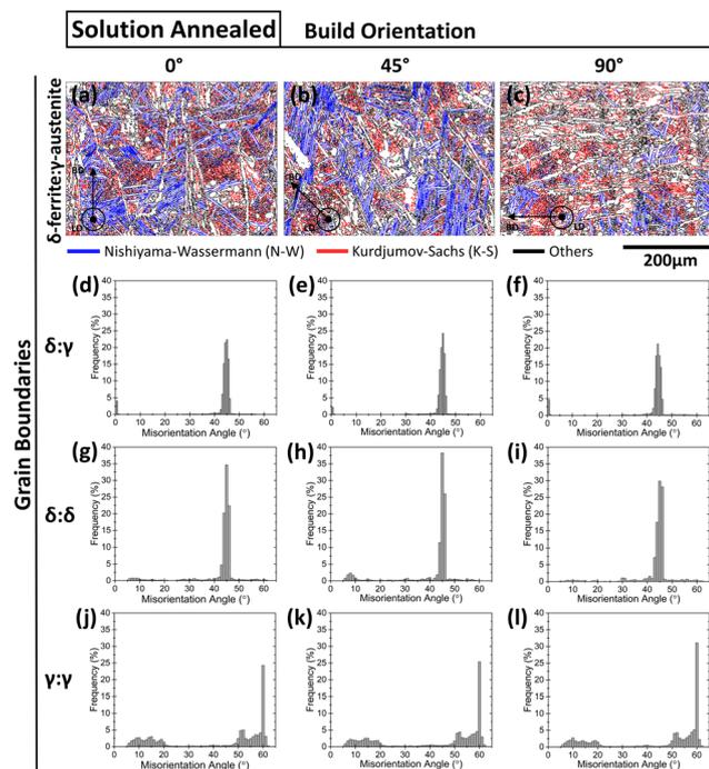
Fig. 12 Solution-annealed samples: (a)–(c) orientation relationships of  $\delta$ -ferrite: $\gamma$ -austenite interfaces; (b) misorientation angle histograms for the (d)–(f)  $\delta$ -ferrite: $\gamma$ -austenite, (g)–(i)  $\delta$ -ferrite: $\delta$ -ferrite and (j)–(l)  $\gamma$ -austenite: $\gamma$ -austenite grain boundaries at each build orientation.
