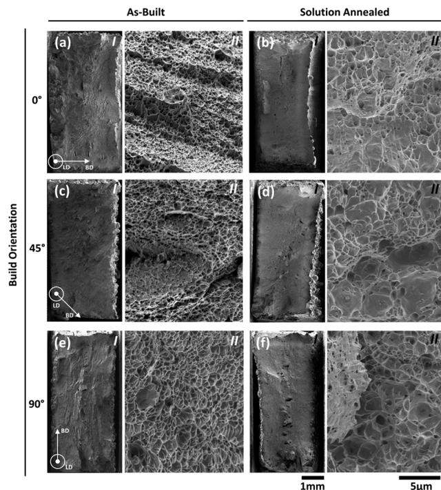
Fig. 19 Fracture surfaces of the as-built and solution-annealed samples in the; (a)–(b) 0°, (c)–(d) 45° and (e)–(f) 90° build orientations at (I) low magnification (35 $\times$ ) and (II) high magnification (5000 $\times$ ).
