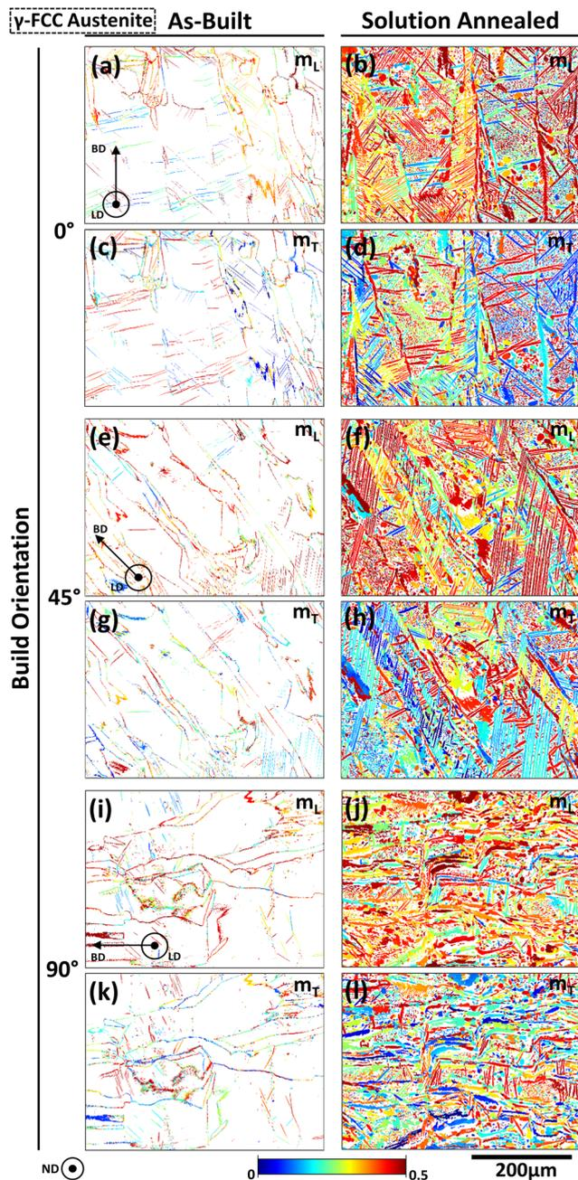
Fig. 17 Schmid factor maps of leading ( $m_L$ ) and trailing ( $m_T$ ) partial dislocations for  $\gamma$ -austenite in the; (a)–(d)  $0^\circ$ , (e)–(h)  $45^\circ$  and (i)–(l)  $90^\circ$  build orientations, taken in the normal direction (ND). The inset denotes the build direction (BD) and loading direction (LD).
