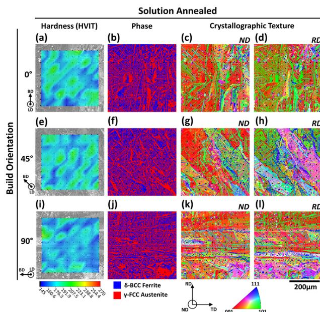
**Fig. 14** Instrumented indentation mapping of solution-annealed samples with corresponding phase, and crystallographic texture maps in the ND and RD, taken in the; (a)–(d)  $0^\circ$ , (e)–(h)  $45^\circ$  and (i)–(l)  $90^\circ$  build orientations.
