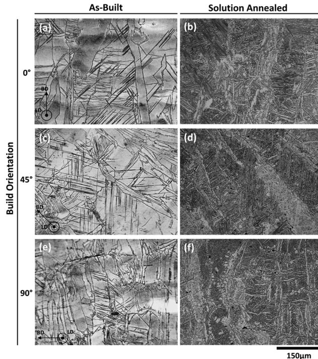
Fig. 5 Cross-sectional micrographs of as-built and solution annealed samples in the; (a)–(b) 0°, (c)–(d) 45° and (e)–(f) 90° build orientations. Inset denotes build direction (BD) and loading direction (LD).
