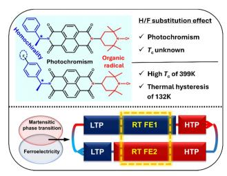
Fig. 14 Effects of H/F substitution in NDI derivatives (top) and the combination of martensitic phase transition and ferroelectricity in S-/R-F NDI derivatives with two different ferroelectric phases at room temperature (bottom). LTP and HTP represent the low-temperature phase and hightemperature phase, respectively. RT FE1 and RT FE2 represent different ferroelectric phases at room temperature (adapted and modified from ref. 132)
