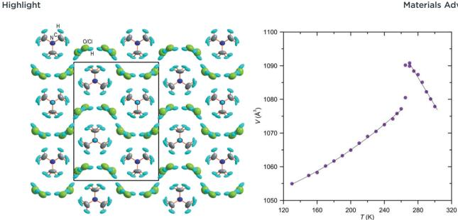
Fig. 18 The crystal structure of the orthorhombic form of dabcoHCl-3H<sub>2</sub>O at 270 K, viewed along [100], showing the H-bonded disordered H<sub>2</sub>O molecules and Cl<sup>-</sup> anions (left). Temperature dependence of the unit-cell volume of dabcoHCl·3H<sub>2</sub>O (right). Reprinted (used in part) from ref. 50.
