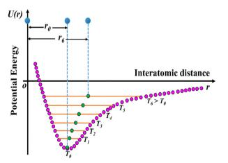
Fig. 3 Schematic diagram of the potential energy well of paired atoms (adapted and modified from ref. 6).
