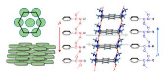
Fig. 12 Schematic illustration of discotic hexacolumnar mesophase (left) and H-bonded 1D columnar structure with dipole ( $\mu$ ) inversion through the collective conformational change of the chain along the  $\pi$ -stacking direction (right). Reprinted (used in part) with permission from ref. 121. Copyright 2015 American Chemical Society.
