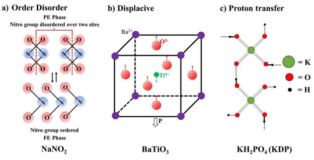
Fig. 5 Different types of mechanisms that lead to the origin of ferroelectricity polarization.
