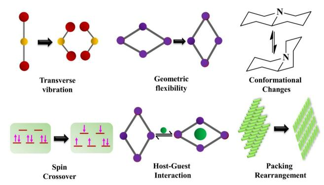
Fig. 15 Various mechanisms leading to negative thermal expansion (NTE) behaviour in molecular materials.
