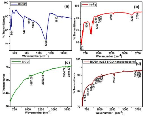
Fig. 2 FTIR spectra of the synthesized NMs (a) BiOBr, (b) In<sub>2</sub>S<sub>3</sub>, (c) SrGO, and (d) the BiOBr-In<sub>2</sub>S<sub>3</sub>-SrGO nanocomposite.
