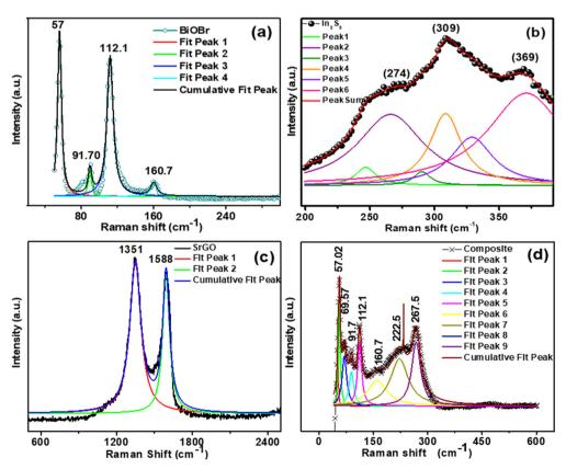
Fig. 3 Raman shift versus intensity of the synthesized NMs (a) BiOBr, (b) In<sub>2</sub>S<sub>3</sub>, (c) SrGO, and (d) the BiOBr-In<sub>2</sub>S<sub>3</sub>-SrGO nanocomposite.
