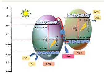
Scheme 1 Mechanism of Cr(vi) reduction using the BiOBr-In<sub>2</sub>S<sub>3</sub>-SrGO
