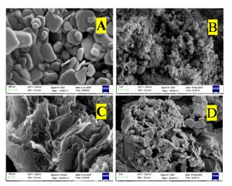
Fig. 5 FE-SEM micrographs of (a) BiOBr, (b) In<sub>2</sub>S<sub>3</sub>, (c) SrGO, and (d) the BiOBr-In<sub>2</sub>S<sub>3</sub>-SrGO nanocomposite.
