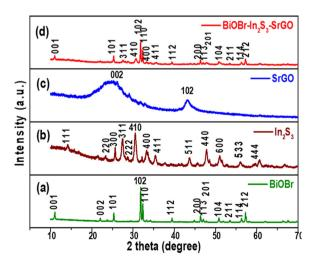
Fig. 1  $\,$  X-ray diffraction patterns of (a) BiOBr, (b) In<sub>2</sub>S<sub>3</sub>, (c) SrGO, and (d) the BiOBr-In<sub>2</sub>S<sub>3</sub>-SrGO nanocomposite.
