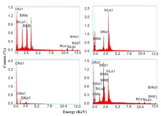
Fig. 6 Energy dispersive X-rays spectrum (EDX) of (a) BiOBr, (b) In<sub>2</sub>S<sub>3</sub>, (c) SrGO, and (d) the BiOBr-In<sub>2</sub>S<sub>3</sub>-SrGO nanocomposite.
