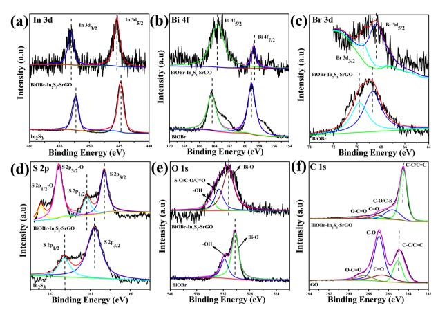
Fig. 8 High-resolution XPS spectra of (a) In 3d, (b) Bi 4f, (c) Br 3d, (d) S 2p, (e) O 1s, and (f) C1s from the bare  $ln_2S_3$ , BiOBr and BiOBr $-ln_2S_3$ -SrGO ternary nanocomposites.
