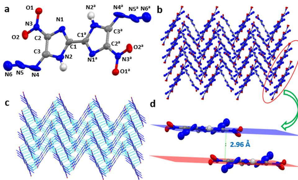
Fig. 2 (a) Crystal structure (water is omitted for clarity). (b) Cross-linked crystal packing along *b*-axis. (c) Non-covalent interactions along *b*-axis (wireframe model). (d) Interlayer distance between two layers for compound **6**.
