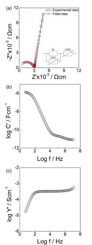
Fig. 5 Impedance data of  $Li_{6.6}La_3ZrNb_{0.8}Zn_{0.2}O_{12}$ . (a) Complex  $Z^*$  plot (b) Spectroscopic plot of C' (c) Spectroscopic plot of Y'.
