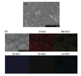
Fig. 4 SEM and EDX elemental mappings of Li<sub>6.6</sub>La<sub>3</sub>ZrNb<sub>0.8</sub>Zn<sub>0.2</sub>O<sub>12</sub>.
