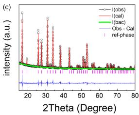
Fig. 2 (a) XRD patterns for  $Li_6La_3ZrNbO_{12}$  and  $Li_{6.6}La_3ZrNb_{0.8}Zn_{0.2}O_{12}$ . (b) Observed, calculated and difference profiles from Rietveld refinement for Li<sub>6</sub>La<sub>3</sub>ZrNbO<sub>12</sub>. (c) Observed, calculated and difference profiles from Rietveld refinement for  $Li_{6.6}La_3ZrNb_{0.8}Zn_{0.2}O_{12}$
