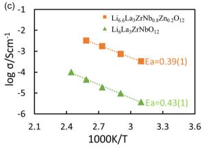
Fig. 6 (a) Arrhenius conductivity plots for  $Li_{5+3x}La_3Nb_{2-x}Zn_xO_{12}$ . (b) Arrhenius conductivity plots for  $Li_{5-2y}Zn_yLa_3Nb_2O_{12}$  (c) Arrhenius conductivity plots for Zn-doped Li<sub>6</sub>La<sub>3</sub>ZrNbO<sub>12</sub>. Unit of activation energy is set as eV.
