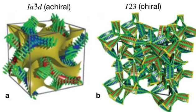
Fig. 1 The two different types of helical network structures of the  $Cub_{bi}$  phases exhibited by the nonsymmetric polycatenars (a) the achiral double-gyroid  $Cub_{bi}/Ia\bar{3}d$  phase and (b) the chiral  $Cub_{bi}^*/I23$  phase, reproduced from ref. 20 by permission from Wiley.
