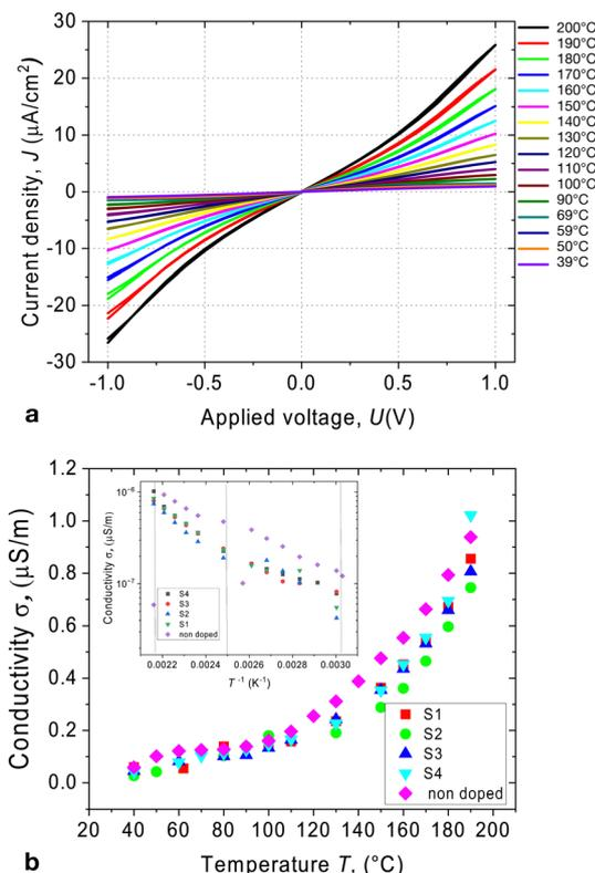
**Fig. 3** (a) The current–voltage characteristic at different temperature of compound **1**. (b) The temperature dependence of conductivity for the pure compound and the mixtures. The inset shows the Arrhenius plot of  $\sigma$ . The measurements were made on non-illuminated samples.
