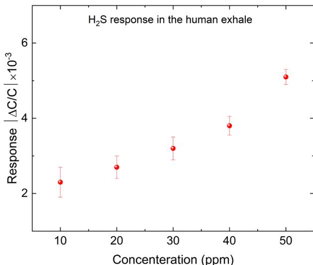
Fig. 6 Response of the sensor to H<sub>2</sub>S in the presence of human exhaled air mixture.
