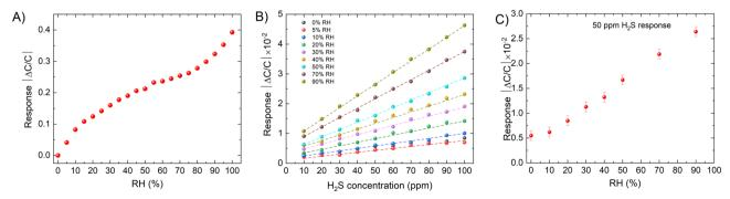
Fig. 5 (A) Response of the kag-MOF to different relative humidity ratios. (B) Response of the sensor to H<sub>2</sub>S in the presence of different RH. (C) Response of the sensor to 50 ppm H<sub>2</sub>S at different relative humidity (RH).
