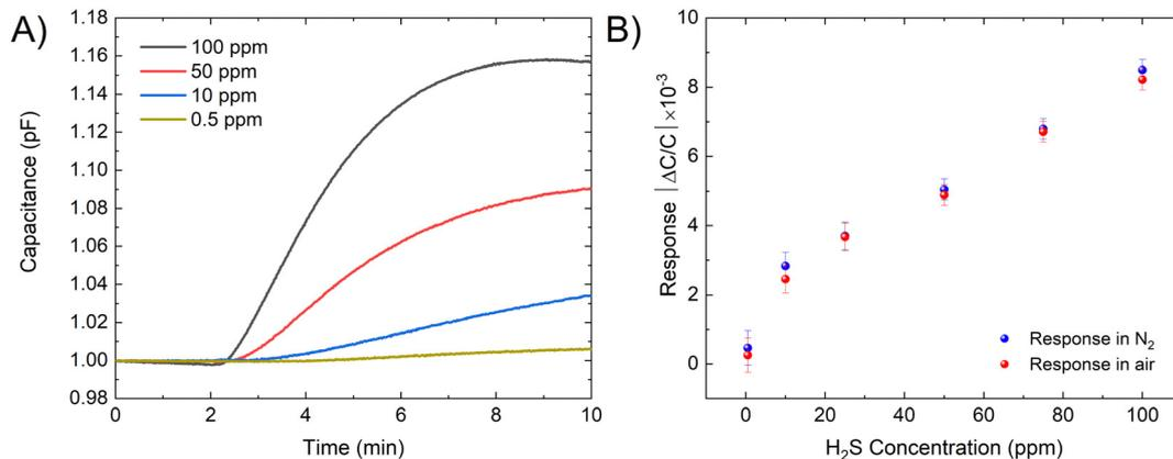
**Fig. 2** (A) Capacitive sensor response for **kag**-MOF in the presence of different concentration of H<sub>2</sub>S. (B) The response of the sensor for different H<sub>2</sub>S concentrations.
