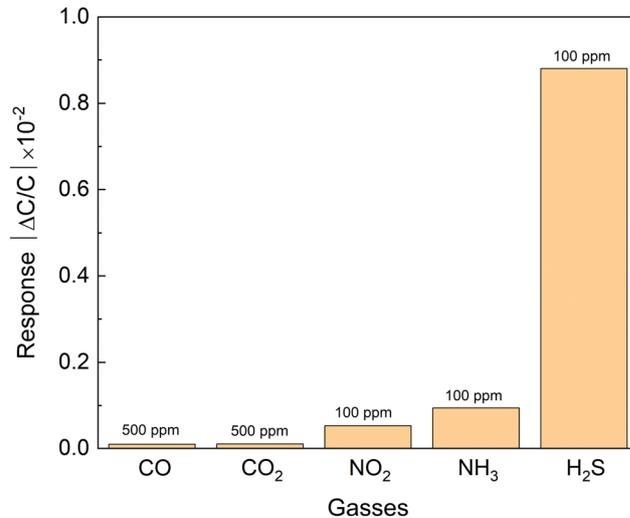
Fig. 4 Selectivity of the **kag**-MOF sensor to hydrogen sulfide (H<sub>2</sub>S), ammonia (NH<sub>3</sub>), nitrogen dioxide (NO<sub>2</sub>), carbon dioxide (CO<sub>2</sub>), and carbon monoxide (CO) at different concentrations.
