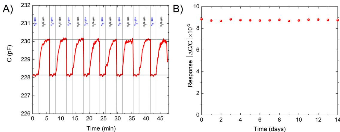
Fig. 3 (A) The recyclability of the sensor in the presence of 100 ppm of H<sub>2</sub>S. (B) The response of the sensor for 100 ppm H<sub>2</sub>S measured daily for 2 weeks.
