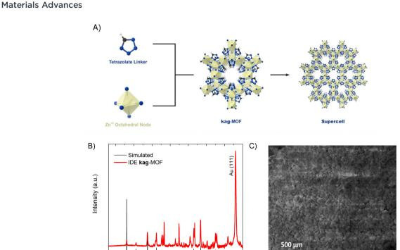
Fig. 1 (A) Simplified schematic representation of the **kag**-MOF showing the channel pore nature and the overall **kag** topology from the supercell. (B) PXRD of the **kag**-MOF film compared with the calculated PXRD from the CIF file. (C) The SEM image of the **kag**-MOF film.
