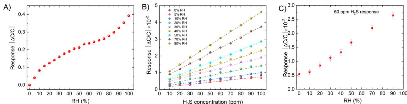
Fig. 5 (A) Response of the **kag**-MOF to different relative humidity ratios. (B) Response of the sensor to H<sub>2</sub>S in the presence of different RH. (C) Response of the sensor to 50 ppm H<sub>2</sub>S at different relative humidity (RH).
