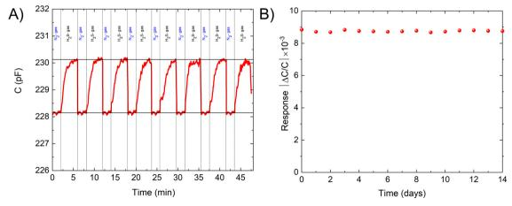
Fig. 3 (A) The recyclability of the sensor in the presence of 100 ppm of H<sub>2</sub>S. (B) The response of the sensor for 100 ppm H<sub>2</sub>S measured daily for 2 weeks.
