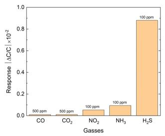
Fig. 4 Selectivity of the kag-MOF sensor to hydrogen sulfide (H2S), ammonia (NH<sub>3</sub>), nitrogen dioxide (NO<sub>2</sub>), carbon dioxide (CO<sub>2</sub>), and carbon monoxide (CO) at different concentrations.
