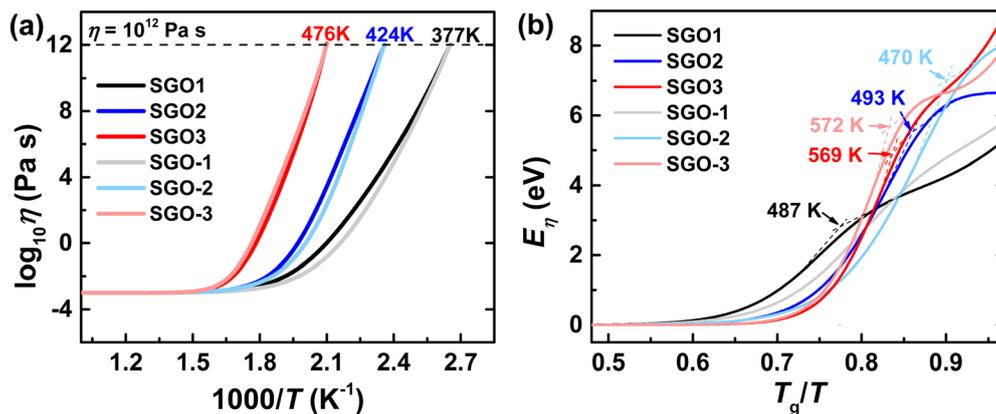
Fig. 7 (a) Angell plots of SGO supercooled liquids. (b) Viscosity activation energy as a function of  $T_g$  scaled temperature,  $E_\eta = k_B \frac{d \ln(\eta/\eta_0)}{d(1/T)}$ , where  $k_B$  is the Boltzmann constant of  $8.617 \times 10^{-5}$  eV  $K^{-1}$  and  $\eta_0$  is a fitted parameter.
