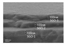
Fig. 1 Cross-sectional view of the SGO multilayer film. The thickness of each SGO phase-change layer is  $\sim 100$  nm and the dielectric layer SiO<sub>2</sub> is  $\sim 5$  nm. Although the 5 nm-thick SiO<sub>2</sub> layer cannot be observed from the SEM pattern directly due to the limited maximum resolution, it can be estimated from the total thickness of this multilayer film.
