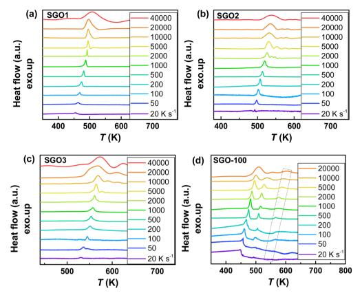
Fig. 4 The representative FDSC traces after background subtraction for (a) SGO1, (b) SGO2, (c) SGO3 single film, and (d) SGO multilayer film. The heating rate is in the range from 20 to 40 000 K s<sup>-1</sup> for single SGO films, and it is in the range from 20 to 20 000 K s<sup>-1</sup> for SGO multilayer films. The black dotted zone in Fig. 4(d) represents the relative weak third-order exothermic peak in the SGO multilayer.
