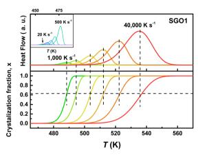
Fig. 6 The JMA numerical simulated FDSC traces (upper layer) and the corresponding crystallized fraction x (bottom layer) of the SGO1 film. The inset in the upper layer depicts the simulated FDSC traces of low heating rates from 20 to 500 K s $^{-1}$ . The horizontal dashed line in the bottom layer indicates the crystallized fraction of 0.63, and the vertical dashed line indicates the  $T_{\rm D}$  at different heating rates.
