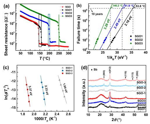
Fig. 3 (a) The temperature-dependent sheet resistances of single SGO films and multilayer SGO film with each phase-change layer is 100 nm. The heating rate is 60 K min<sup>-1</sup>. (b) The Arrhenius plots of three single SGO films. (c) The Kissinger plots of each SGO phase-change layer in multilayer SGO films. (d) The XRD patterns of crystalline states for single SGO films and each phase-change layer in multilayer SGO film.
