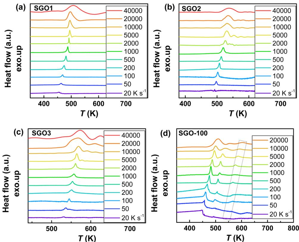
Fig. 4 The representative FDSC traces after background subtraction for (a) SGO1, (b) SGO2, (c) SGO3 single film, and (d) SGO multilayer film. The heating rate is in the range from 20 to 40 000  $\text{K s}^{-1}$  for single SGO films, and it is in the range from 20 to 20 000  $\text{K s}^{-1}$  for SGO multilayer films. The black dotted zone in Fig. 4(d) represents the relative weak third-order exothermic peak in the SGO multilayer.
