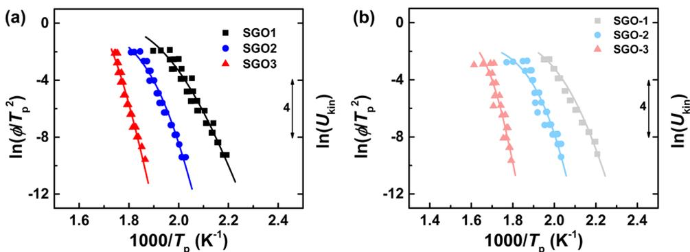
Fig. 5 (a) The Kissinger plots of three single SGO films. (b) The Kissinger plots of each phase-change layer in multilayer SGO film. The related  $U_{\text{kin}}$  of these SGO films are extrapolated as curved lines using eqn (3).
