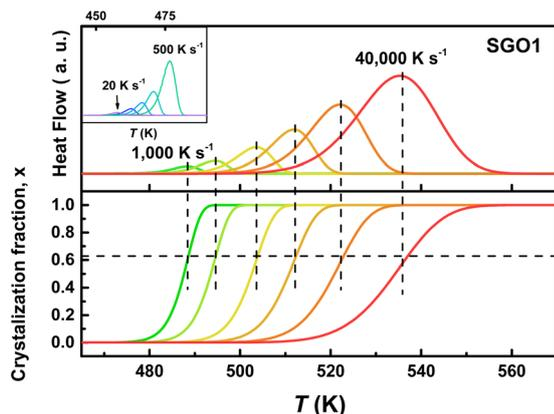
Fig. 6 The JMA numerical simulated FDSC traces (upper layer) and the corresponding crystallized fraction  $x$  (bottom layer) of the SGO1 film. The inset in the upper layer depicts the simulated FDSC traces of low heating rates from 20 to 500 K s<sup>-1</sup>. The horizontal dashed line in the bottom layer indicates the crystallized fraction of 0.63, and the vertical dashed line indicates the  $T_p$  at different heating rates.
