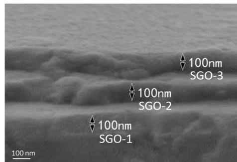
Fig. 1 Cross-sectional view of the SGO multilayer film. The thickness of each SGO phase-change layer is  $\sim 100$  nm and the dielectric layer SiO<sub>2</sub> is  $\sim 5$  nm. Although the 5 nm-thick SiO<sub>2</sub> layer cannot be observed from the SEM pattern directly due to the limited maximum resolution, it can be estimated from the total thickness of this multilayer film.
