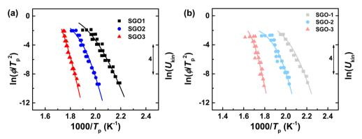
Fig. 5 (a) The Kissinger plots of three single SGO films. (b) The Kissinger plots of each phase-change layer in multilayer SGO film. The related Ukin of these SGO films are extrapolated as curved lines using egn (3).
