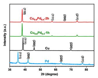
Fig. 2 Overlaid XRD patterns of monometallic Pd, Cu and binary Cu<sub>0.6</sub>Pd<sub>0.4</sub> alloy films prepared via the AACVD process.
