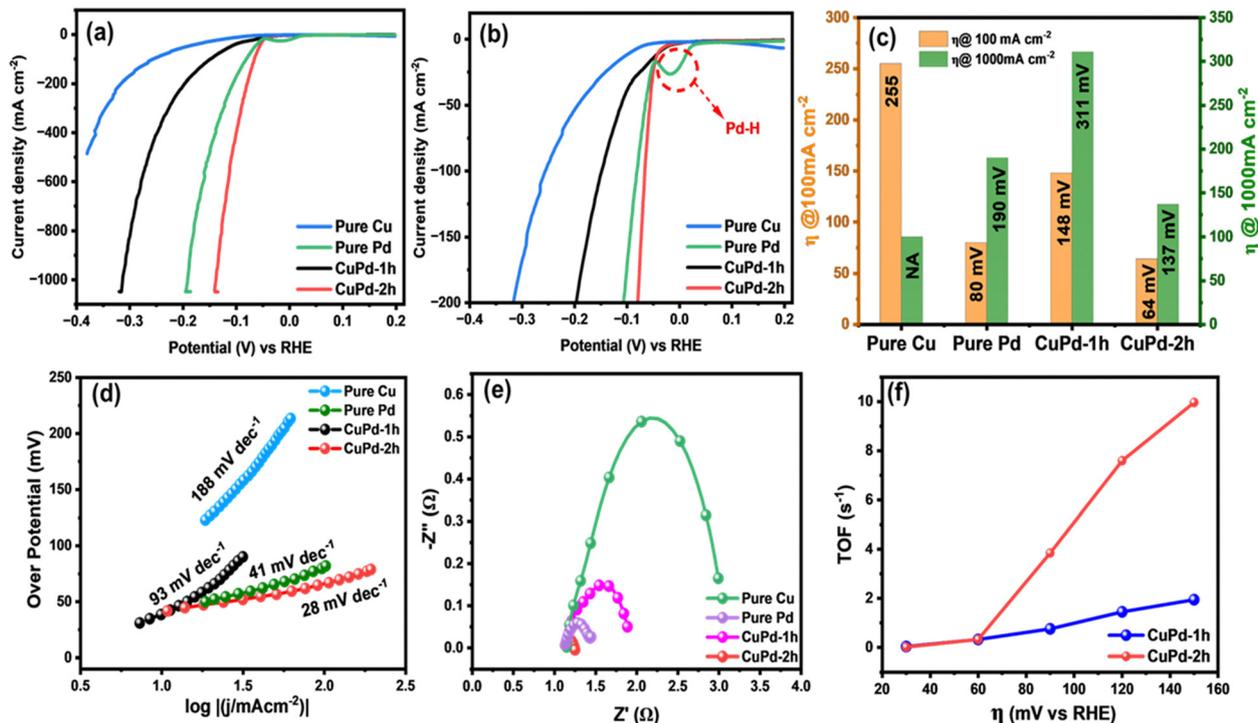
Fig. 6 Electrochemical HER measurements of different electrocatalysts in 0.5 M H<sub>2</sub>SO<sub>4</sub> solution. LSV curves (a), enlarged LSV curves (b), overpotential ( $\eta$ ) comparison at different current densities of 100 and 1000 mA cm<sup>-2</sup> (c), Tafel slopes derived from the corresponding LSV curves (d), EIS Nyquist plots (e), and turnover frequency (TOF) curves (f).
