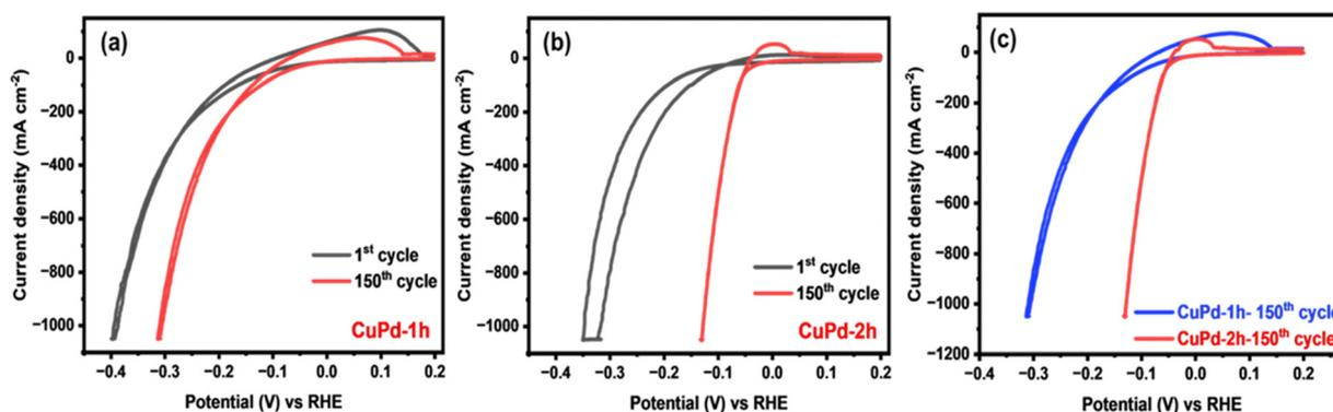
Fig. 5 CV analysis of binary CuPd alloy electrocatalysts performed at a scan speed of  $50 \text{ mV s}^{-1}$  in  $0.5 \text{ M H}_2\text{SO}_4$  electrolyte deposited for 1 h (a) and 2 h (b) and comparison of the 150th CV curves of both alloy samples (c).
