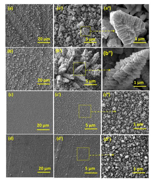
Fig. 3 SEM images captured at different resolutions; binary CuPd alloy deposited for 1 h (a) and 2 h (b). Monometallic Cu (c) and Pd (d) grown on a graphite substrate.
