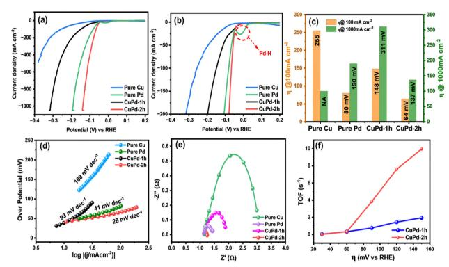
Fig. 6 Electrochemical HER measurements of different electrocatalysts in 0.5 M H<sub>2</sub>SO<sub>4</sub> solution. LSV curves (a), enlarged LSV curves (b), overpotential (η) comparison at different current densities of 100 and 1000 mAcm<sup>-2</sup> (c), Tafel slopes derived from the corresponding LSV curves (d), EIS Nyquist plots (e), and turnover frequency (TOF) curves (f).
