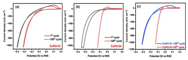
Fig. 5 CV analysis of binary CuPd alloy electrocatalysts performed at a scan speed of 50 mV s<sup>-1</sup> in 0.5 M  $H_2SO_4$  electrolyte deposited for 1 h (a) and 2 h (b) and comparison of the 150th CV curves of both alloy samples (c).
