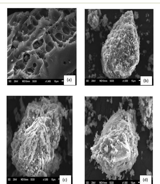
Fig. 3 Micrographs of CP (a) and geoadsorbents GP<sub>0</sub> (b), GP<sub>7.5-CP</sub> (c) and GP<sub>10-CP</sub> (d).
