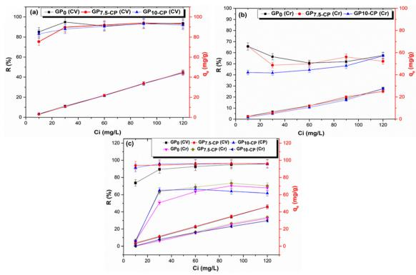
Fig. 7 Effect of initial concentration on single (a), (b) and binary (c) adsorption of CV and  $Cr(v_1)$  on geomaterials. Experimental conditions ( $m_{GP} = 0.1 \, \text{g}$ ,  $V = 0.1 \, \text{g}$ , V =40 mL, T = 25  $\pm$  1  $^{\circ}$ C and t = 60 min).
