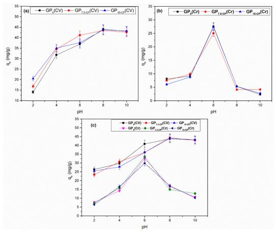
Fig. 5 Influence of pH in single (a), (b) and binary (c) retention of CV and Cr(vi) on geomaterials. Experimental conditions ( $m_{GP} = 0.1 \text{ g}$ , V = 40 mL,  $T = 25 \pm 1 \,^{\circ}\text{C}$ ,  $C_i = 120 \text{ mg L}^{-1}$  and t = 60 min).
