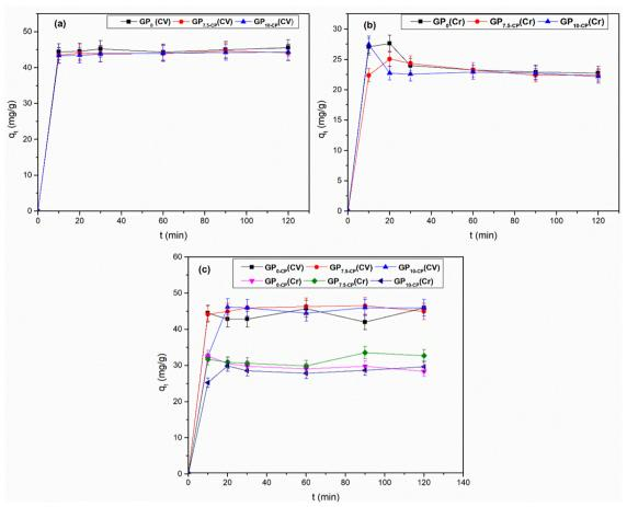
Fig. 6 Effect of contact time on CV and Cr(vi) fixation performance of geomaterials in single (a), (b) and binary (c) systems. Experimental conditions  $(m_{\rm GP} = 0.1 \text{ g}, V = 40 \text{ mL}, T = 25 \pm 1 \,^{\circ}\text{C} \text{ and } C_{\rm i} = 120 \text{ mg L}^{-1}).$
