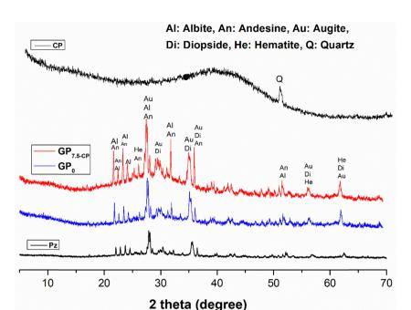
Fig. 1 PXRD patterns of raw material (CP and Pz) and geomaterial (GP<sub>0</sub> and GP<sub>7,5-CP</sub>)
