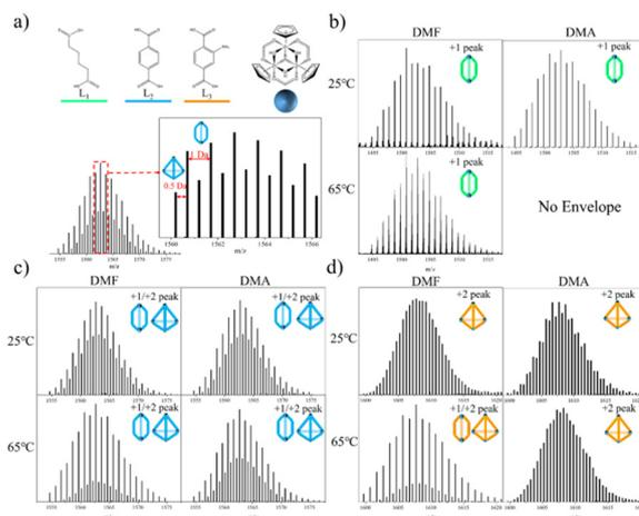
Fig. 1 (a) Bridging linker,  $\text{L}_1$ ,  $\text{L}_2$ ,  $\text{L}_3$ , zirconium cluster and determination of cigar and tetrahedron. (b) ESI-Q-TOF analysis of Zr-MOCs with  $\text{L}_1$ . (c) ESI-Q-TOF analysis of Zr-MOCs with  $\text{L}_2$ . (d) ESI-Q-TOF analysis of Zr-MOCs with  $\text{L}_3$ .
