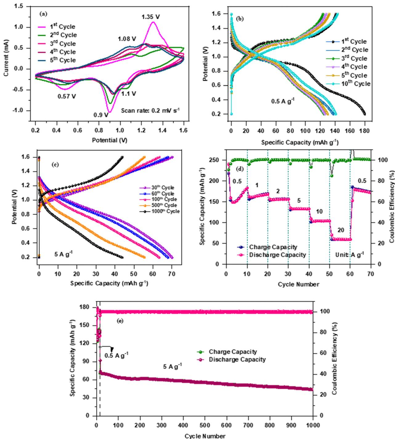
Fig. 3 (a) Cyclic voltammograms at a constant scan rate of  $0.2 \text{ mV s}^{-1}$ ; (b) discharge/charge curves at a current density of  $0.5 \text{ A g}^{-1}$  for the initial five cycles; (c) discharge/charge curves at a current density of  $5 \text{ A g}^{-1}$  for 1000 cycles; (d) C-rate performance at different current densities and (e) cycling performance at a constant current density of  $5 \text{ A g}^{-1}$  until 1000 cycles of the nanoplate-shaped  $\text{V}_2\text{O}_5$  electrode.
