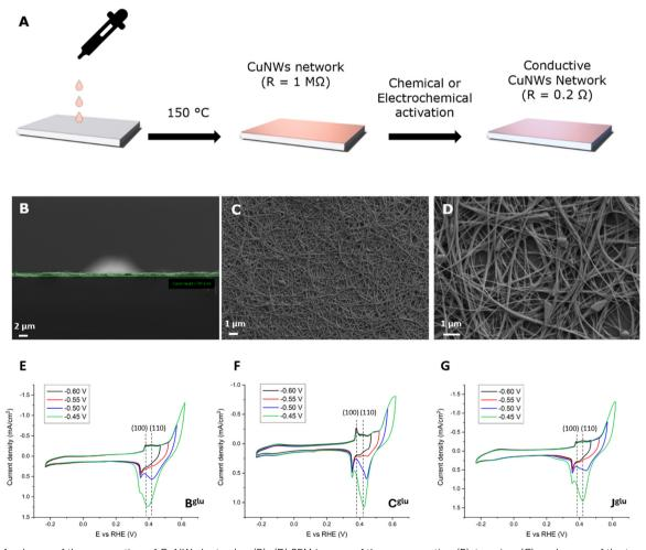
Fig. 4 (A) A scheme of the preparation of CuNW electrodes. (B) – (D) SEM images of the cross-section (B), top view (C), and zoom of the top view (D) of CuNW electrodes. (E) Cyclic voltammetry in 1 M NaOH recorded for B<sup>glu</sup> (E), C<sup>glu</sup> (F), and J<sup>glu</sup> (G) CuNW electrodes. Inverting the potential at different values, the effect of different degrees of Cu(ı) oxidation on the voltametric pattern. The vertical dotted lines assign the peaks to crystal facets.
