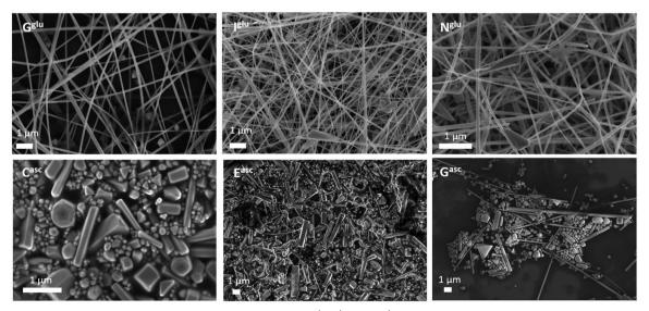
Fig. 2 Representative SEM images from the glucose synthesis route, G<sup>glu</sup>, I<sup>glu</sup>, and N<sup>glu</sup>, and from the sodium ascorbate synthesis route, C<sup>asc</sup>, E<sup>asc</sup>, and Gasc.
