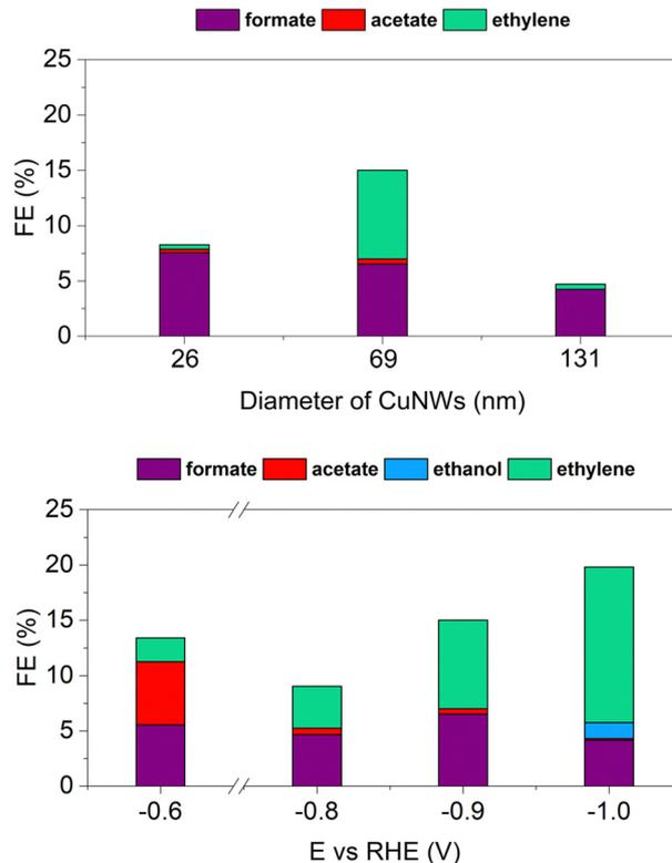
Fig. 5 (A) Faradaic efficiency of three different CuNWs,  $\text{B}^{\text{glu}}$ ,  $\text{C}^{\text{glu}}$ , and  $\text{J}^{\text{glu}}$ , at  $-0.9$  V *vs.* RHE in 1 M  $\text{KHCO}_3$  solution. (B) Faradaic efficiency of  $\text{C}^{\text{glu}}$  at different electrochemical potentials in 1 M  $\text{KHCO}_3$ .
