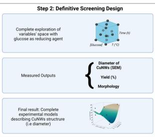
Fig. 1 Workflow to establish the relationship between the synthesis parameters and the morphology of CuNWs, based on a sequential DOE approach.
