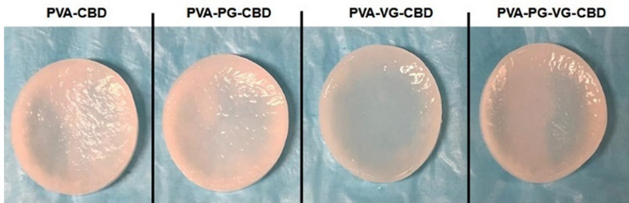
Fig. 1 CBD-rich hydrogels produced through 8 freeze–thaw cycles. The softness, slight elasticity and toughness make the hydrogels can be comfortably handled. The uniform distribution of CBD renders the hydrogels pinkish.
