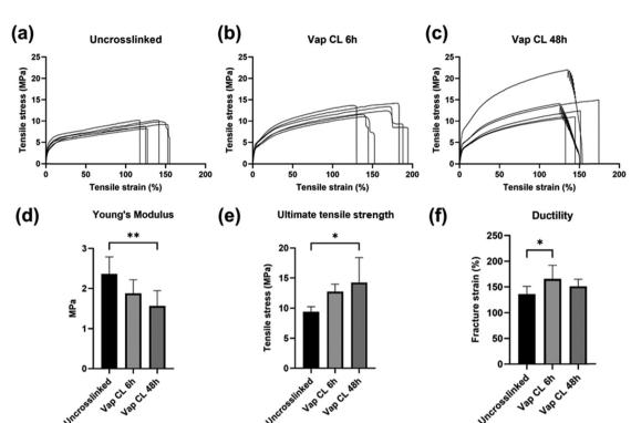
Fig. 4 Mechanical properties of uncrosslinked, vapour and *in situ* crosslinked electrospun meshes. (a)—(c) Stress—strain curves of uncrosslinked, Vap CL 6 h and Vap CL 48 h, (d) Young's modulus, (e) ultimate tensile strength and (f) ductility of the same meshes.
