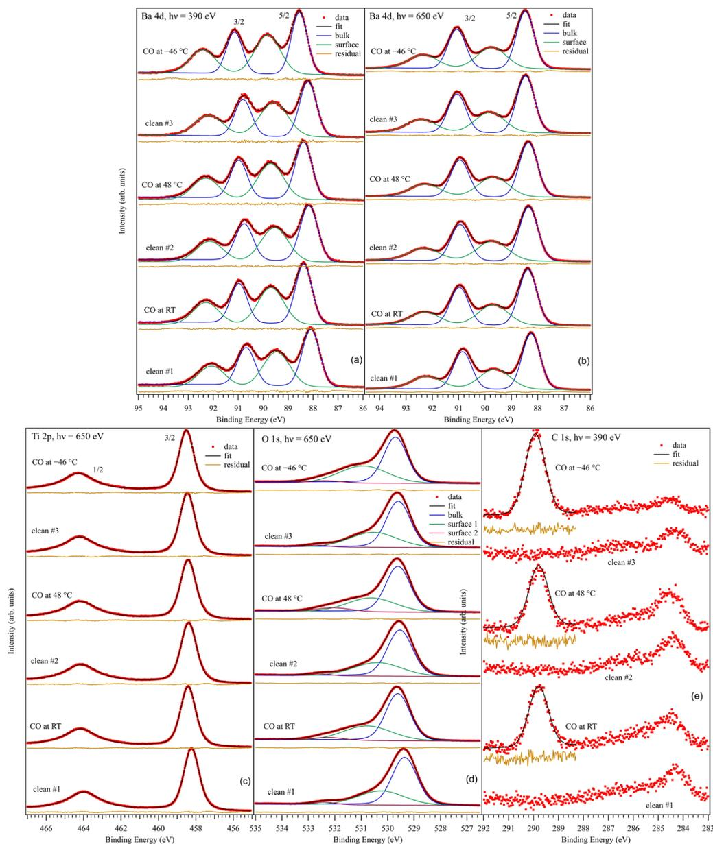
Fig. 3 Core level X-ray photoelectron spectroscopy for Ba 3d (a) and (b), Ti 2p (c), O 1s (d) and C 1s (e) for BaTiO<sub>3</sub>(001) clean and after several doses with 3.4 kL CO at different temperatures. The employed photon energies are specified on each graph.
