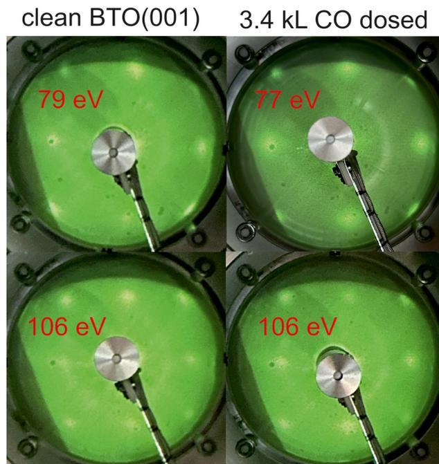
Fig. 2 Low energy electron diffraction (LEED) images on clean BaTiO<sub>3</sub>(001) and after CO dosing. The electron energies are indicated on each photograph.
