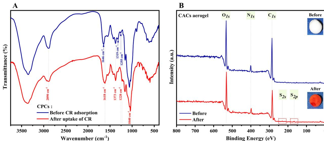
Fig. 11 (A) FTIR and, (B) XPS survey spectra of CPCs aerogel before (blue line) and after (red line) CR adsorption (initial concentration of 1000 mg L<sup>-1</sup>) at pH = 7.4.
