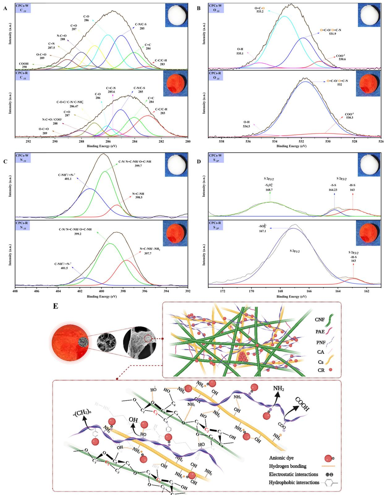
Fig. 12 High-resolution XPS spectra of (A)  $C_{1s}$ , (B)  $O_{1s}$ , (C)  $N_{1s}$ , and (D)  $S_{2p}$  of CPCs aerogel before and after CR adsorption at pH = 7.4, (CPCs-W, the inset image indicates the white CPCs aerogel bead as control sample) (CPCs-R, the inset image represents the aerogel bead after adsorption), (E) schematic representation of the binding of CR on to the CPCs aerogel surface.
