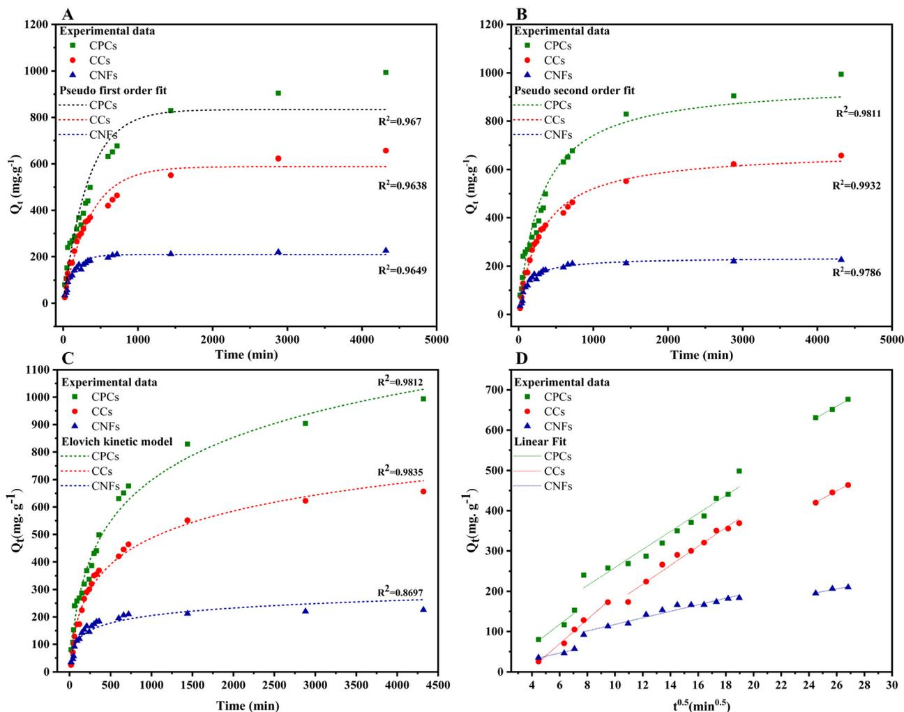
Fig. 9 Kinetic modelling of the adsorption of CR dye (initial concentration of  $1000 \text{ mg L}^{-1}$ ) onto the aerogels with various compositions, *i.e.*, single-component (CNFs), hybrid (CCs), and three-component (CPCs) aerogel composite beads: (A) Pseudo-first-order, (B) Pseudo-second-order, (C) Elovich, (D) intraparticle diffusion models.
