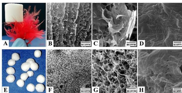
**Fig. 2** Comparing two distinct freeze-casting techniques: (A) the digital photo of cylindrical CPCs aerogel prepared through unidirectional freezing technique, standing on top of a feather. (B) FE-SEM image, (C) and (D) high-resolution FE-SEM images of the cylindrical composite aerogel. (E) Digital photo of highly porous CPCs aerogel beads prepared by radial-freezing technique. (F) FE-SEM image, (G) and (H) high-resolution FESEM images of the CPCs aerogel bead.
