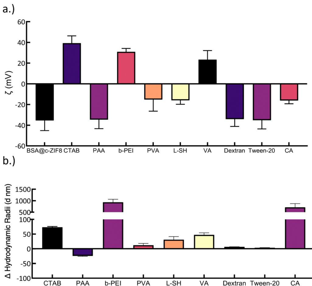
Fig. 5 Average hydrodynamic radius and  $\zeta$  potential of BSA@c-ZIF-8 after surface passivation. (a)  $\zeta$  potential of BSA@c-ZIF-8 before and after surface passivation with various polymers and ligands. (b)  $\Delta$  hydrodynamic radii (d nm) of polymer coated BSA@c-ZIF-8 relative to uncoated BSA@c-ZIF-8. Each bar and error represents the average standard deviation across three batches, each measured thrice ( $n = 9$ ).
