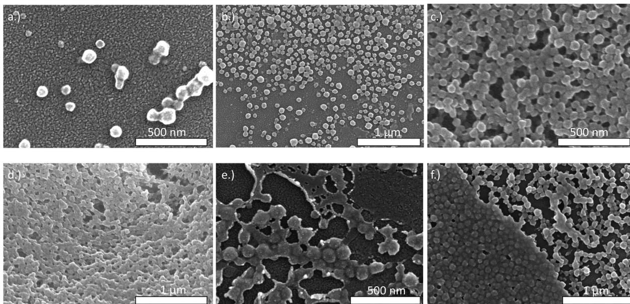
Fig. 3 SEM images of BSA@c-ZIF-8 after incubating in buffer for 24 h. The buffers used are as follows; (a) water, (b) PBS (pH 7.1), (c) IM buffer (pH 7.5), (d) HEPES buffer (pH 7.4), (e) MES buffer (pH 6.0), and (f) MOPS (pH 7.2).
