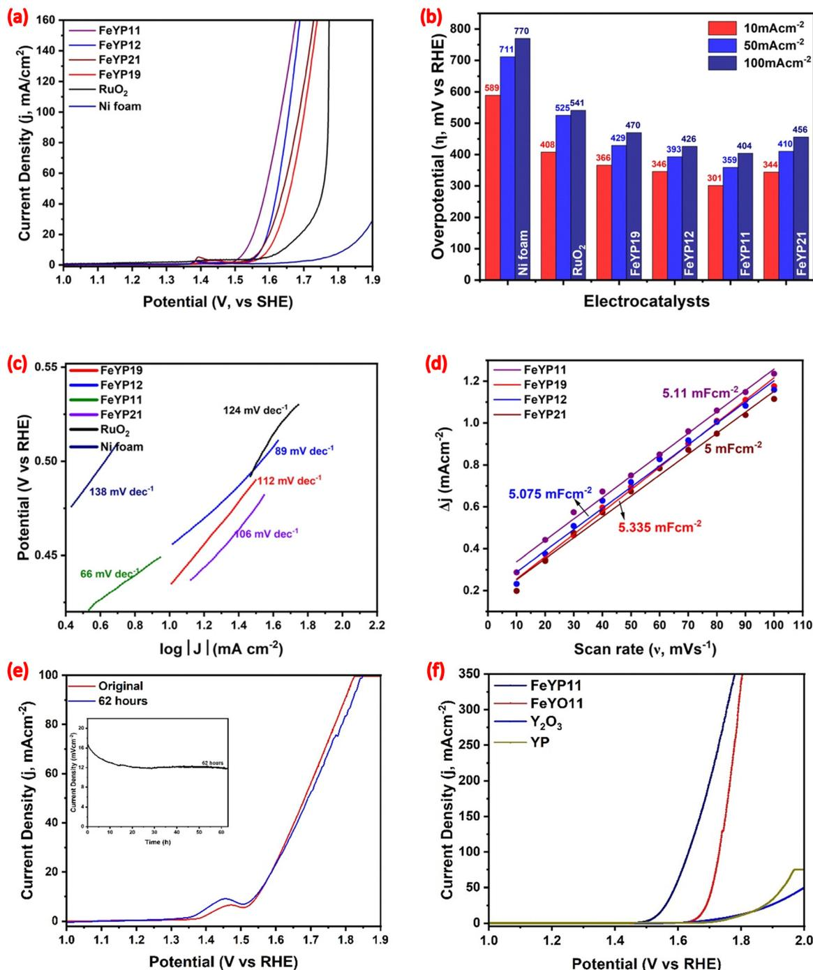
Fig. 4 OER performance of the prepared samples. (a) Polarization curves in a 1 M KOH solution (with 100% iR correction)<sup>38</sup> at a potential window of 0.9 V to 2 V with a scan rate of 10 mV s<sup>-1</sup>, (b) comparative bar diagrams of overpotential at different current densities, (c) Tafel plots, (d) double-layer capacitance measurements, (e) the chronopotentiometry curve of Fe-YP11 in 1 M KOH, and (f) polarization curves of FeYP11, FeYO11, Y<sub>2</sub>O<sub>3</sub> and YP.
