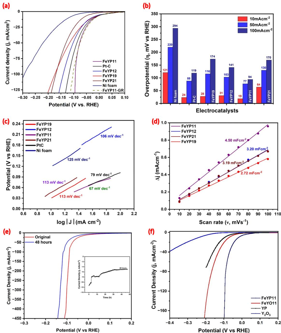
Fig. 5 HER performance of the as-prepared samples. (a) Polarization curves at a 10 mV s<sup>-1</sup> scan rate, (b) comparative bar diagrams of overpotential at different current densities, (c) Tafel plots, (d) double-layer capacitance measurements, (e) the chronopotentiometry curve of FeYP11, and (f) polarization curves of FeYP11, FeYO11, YP and Y<sub>2</sub>O<sub>3</sub> in 1 M KOH solution.
