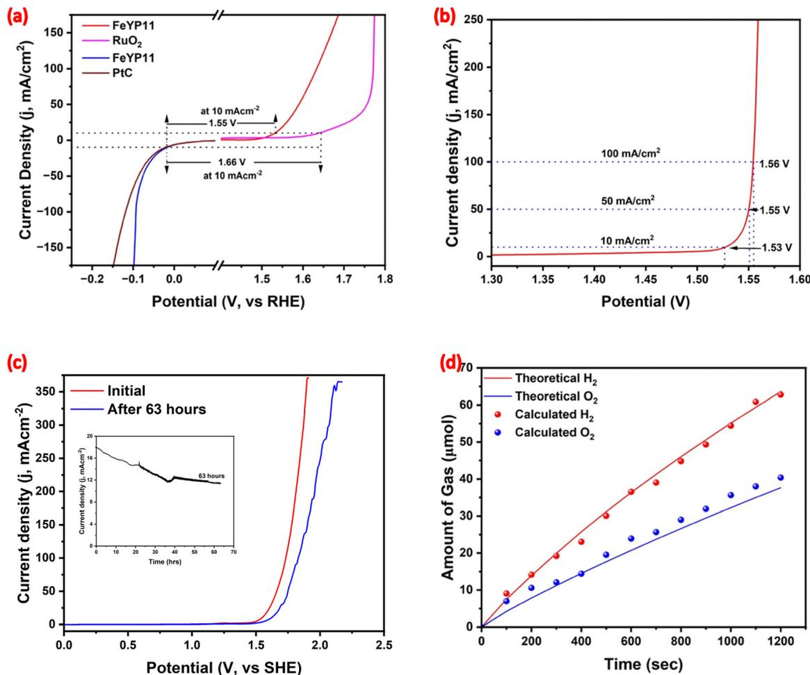
Fig. 6 (a) Half-cell HER and OER polarization curves at a scan rate of  $10 \text{ mV s}^{-1}$ , (b) polarization curves of FeYP11 (+)//FeYP11 (–) in a two-electrode system, (c) two-electrode measurements for overall water-splitting performance for 60 hours, and (d) amount of  $\text{H}_2$  and  $\text{O}_2$  gas evolved at a constant overpotential of 406 mV.
